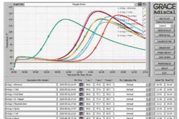
Fig. 3: Adiacal evaluations of the effects of regular soft drink (with sugar) additions on temperature development in mortar mixtures
