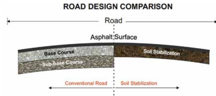
Fig. 2: Conventionally constructed road versus AggreBind RM1 stabilized road
