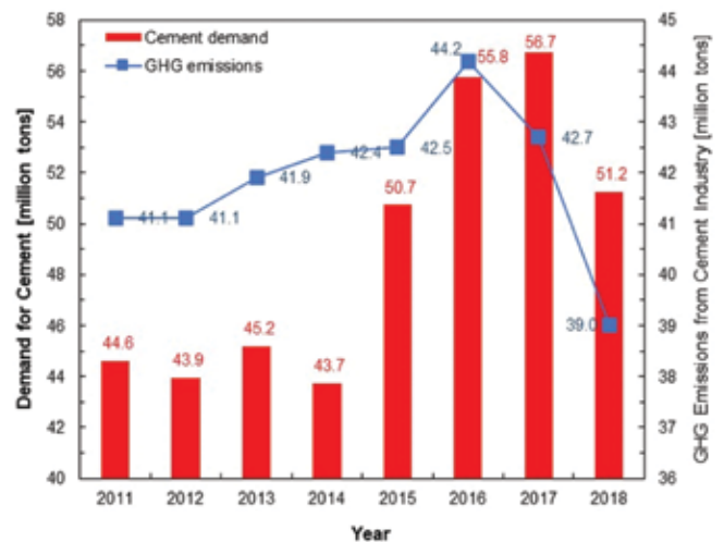
Fig. 1: Cement demand and greenhouse gas (GHG) emissions from the cement industry in South Korea (Note: 1 tonne = 1.1 ton)
