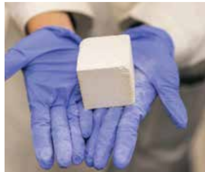
Mortar cube sample made with ReAct green cement
