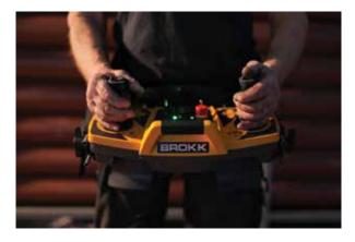
hand while simultaneously monitoring the status of the machine. A two-way communication system communicates the status back to the operator in real time, while customized features enhance the operating experience. SmartPower+ also alerts the operator about any unwanted power supply or machine statuses, further contributing to an increase in uptime and reliability.
