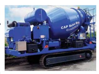
on wheels or trucks. Factory options include soundproofing for work in densely populated urban areas, a hopper screen vibrator for harsh mixtures, and an automatic lubrication system.
