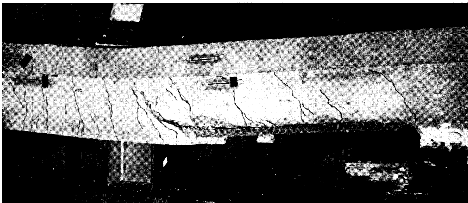
Fig. 3—Typical shear-tension failure
