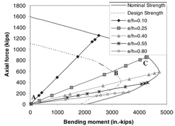
Fig. 4—P-M interaction diagram and loading histories for typical column ( $\rho_g = 1\%$  and  $f'_c = 4000$  psi).
