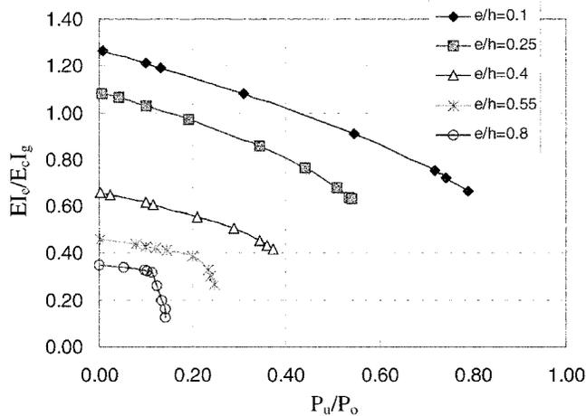
Fig. 6—Influence of eccentricity ratio and axial load ratio on effective  $I$  of columns ( $\rho_g = 1\%$  and  $f'_c = 4000$  psi).
