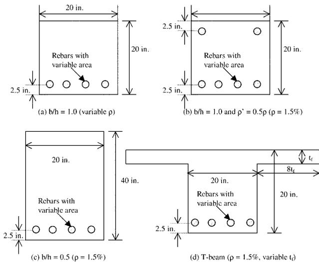
Fig. 8—Cross section of typical reinforced concrete beams considered in parametric study.
