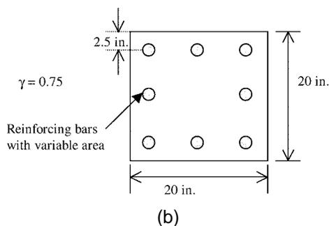
Fig. 2—(a) Moment-curvature relationship for typical reinforced concrete column considered in parametric study (for  $e/h$  ratio of 0.25 and reinforcement ratio of 3%); and (b) cross section of typical reinforced concrete column considered in parametric study.
