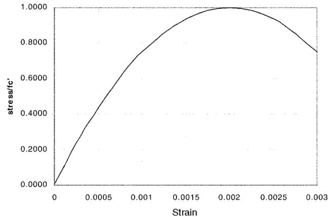
Fig. 5—Typical stress-strain curve for concrete in compression.
