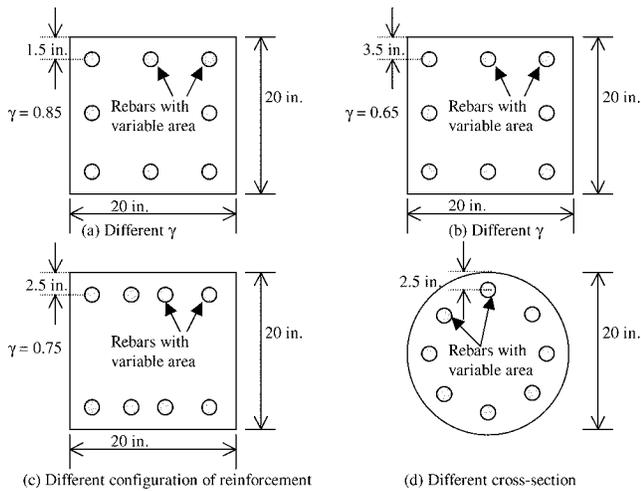
Fig. 3—Cross section of typical reinforced concrete columns considered in parametric study.
