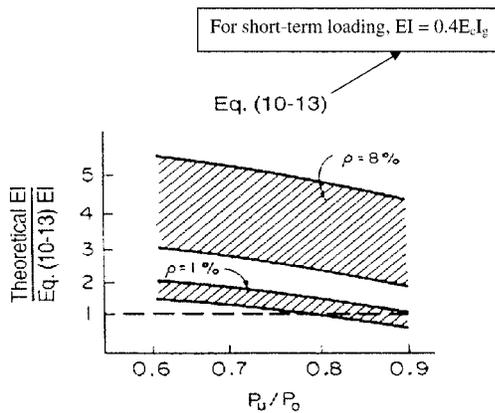
Fig. 11—Comparison of ACI 318-95, Eq. (10-13) (same as Eq. (10-12) in ACI 318-02) for EI with EI values from moment-curvature diagrams (MacGregor, Breen, and Pfrang 1970).
