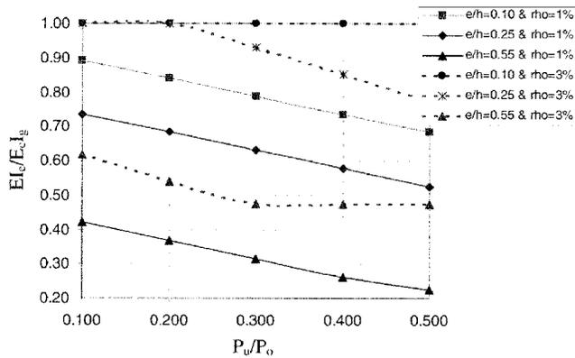
Fig. 12—Influence of axial load and eccentricity ratio on flexural stiffness of columns.
