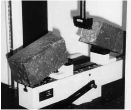
Fig. 6 Failure mode of the prismatic specimens in bending.
