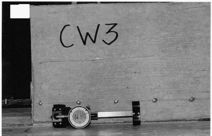
Fig. 13. DEMEC strain gauge and targets.
