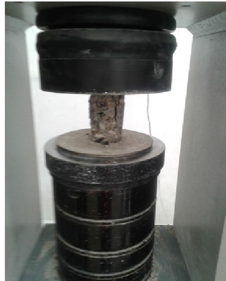
Fig. 22 Crushing core concrete.
