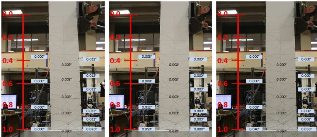
Figure C-6: Measured Crack Widths at Drift Ratio of 1.75% – Specimen SBH60
