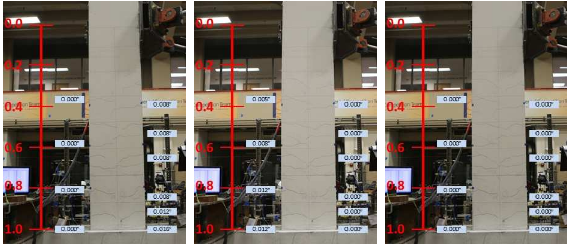
Figure C-3: Measured Crack Widths at Drift Ratio of 0.6% – Specimen SBH60
