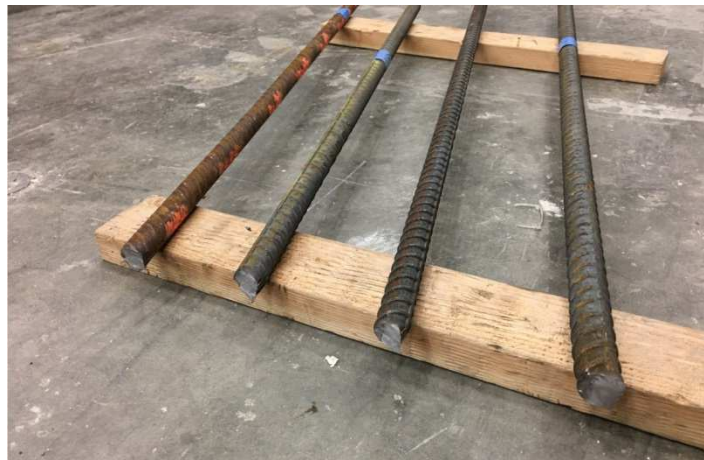
Figure A-5: Longitudinal Steel Used in Test Specimens - Left to Right: SBL100, SBH100, SBM100, SBH60
