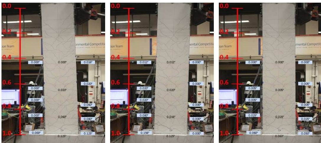
Figure C-28: Measured Crack Widths at Drift Ratio of 3.45% – Specimen SBM100
