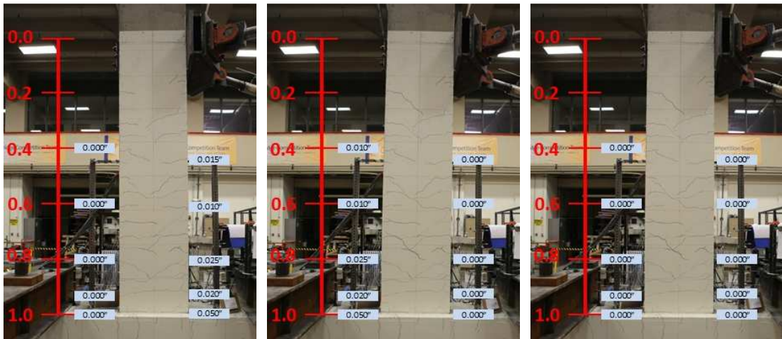
Figure C-18: Measured Crack Widths at Drift Ratio of 1.25% – Specimen SBL100
