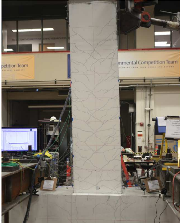
Figure 3.1.4: Deflected shape of SBM100 at Drift Ratio 2.45% (Left) and 3.45% (Right).
