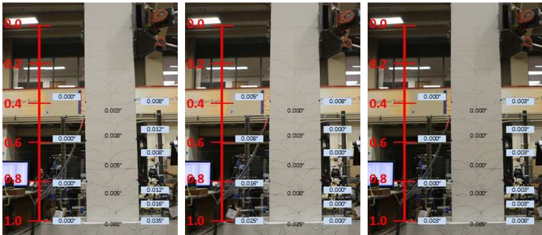
Figure C-4: Measured Crack Widths at Drift Ratio of 0.9% – Specimen SBH60
