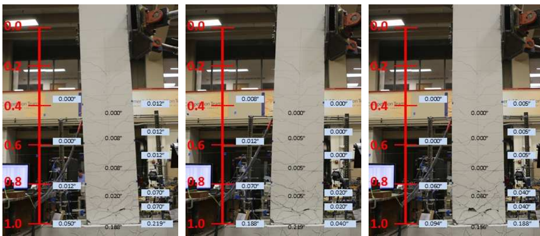
Figure C-8: Measured Crack Widths at Drift Ratio of 3.45% – Specimen SBH60
