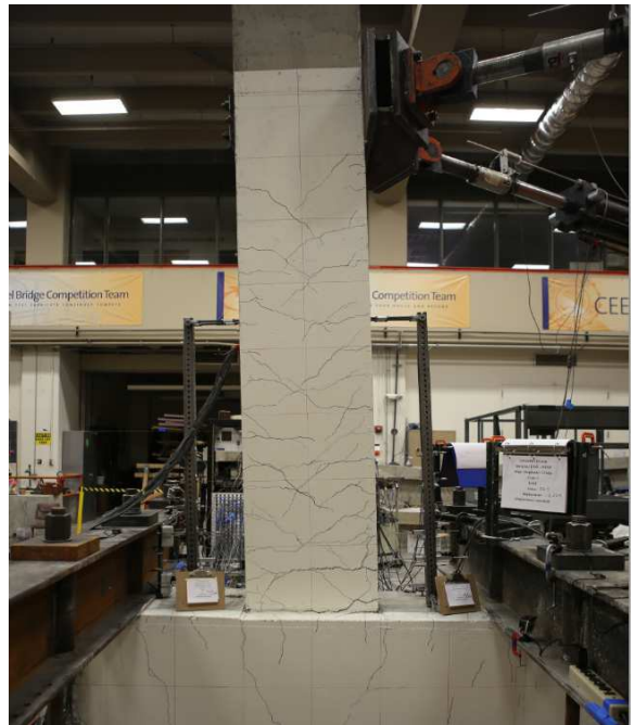
Figure 3.1.3: Deflected shape of SBL100 at Drift Ratio 2.45% (Left) and 3.45% (Right).
