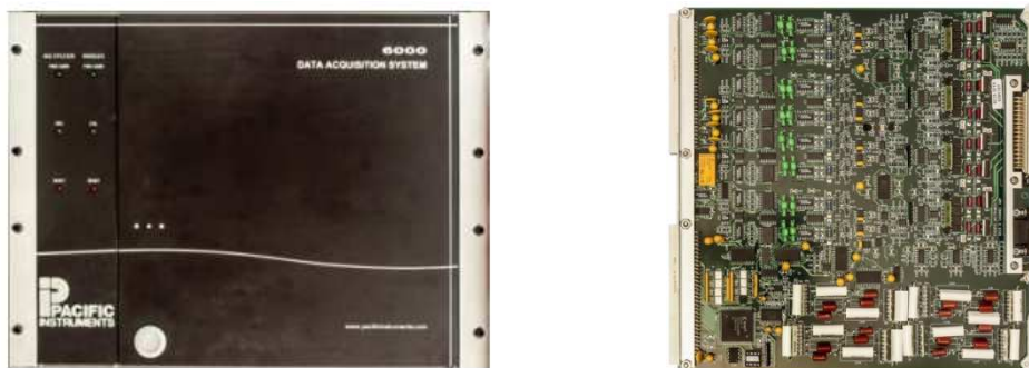
Figure A-25: Left: Data Acquisition System; Right: Analog I/O Modules
