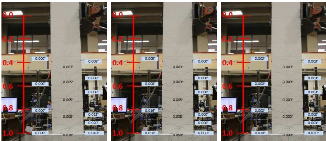
Figure C-5: Measured Crack Widths at Drift Ratio of 1.25% – Specimen SBH60
