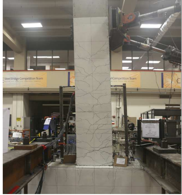
Figure 3.1.2: Deflected shape of SBH100 at Drift Ratio 2.45% (Left) and 3.45% (Right).
