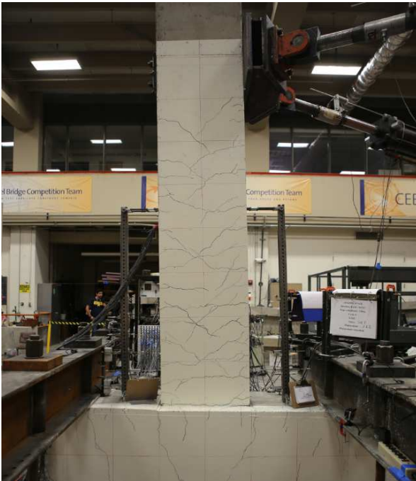
Figure 3.1.3: Deflected shape of SBL100 at Drift Ratio 2.45% (Left) and 3.45% (Right).
