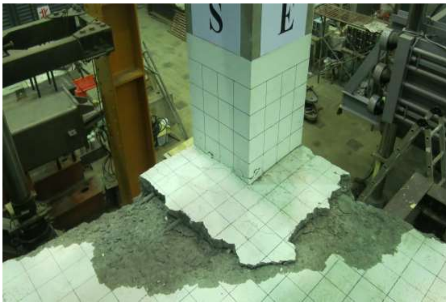
(b) After Loose Concrete Removal
