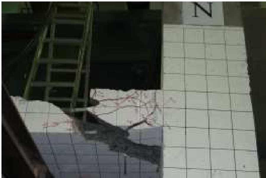
(b) After Loose Concrete Removal
