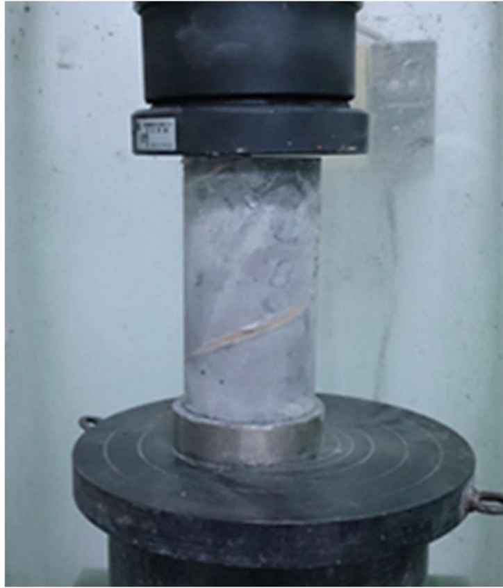
Fig. 4.2 – Concrete Compressive Strength Testing
