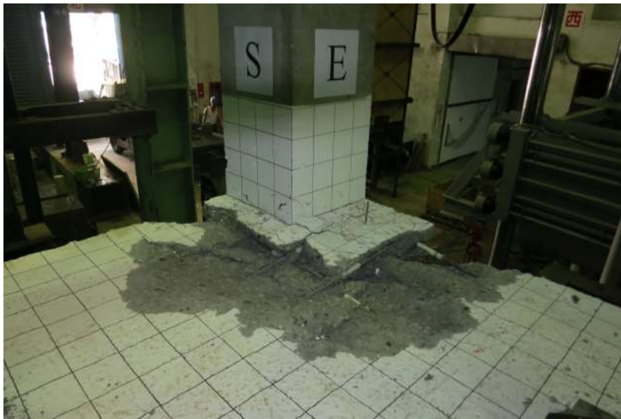
(b) After Loose Concrete Removal
