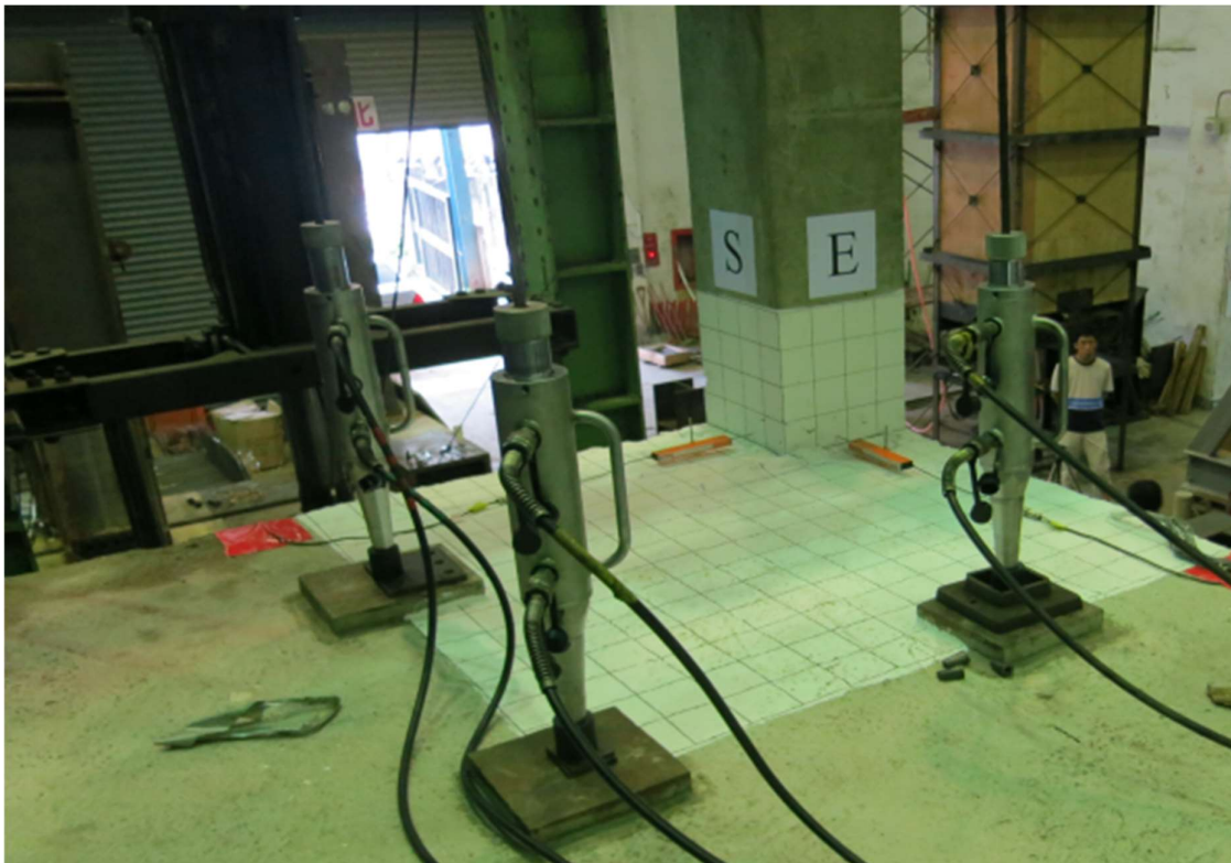
Fig. 3.14 – Hydraulic Jacks for Gravity Loading Application
