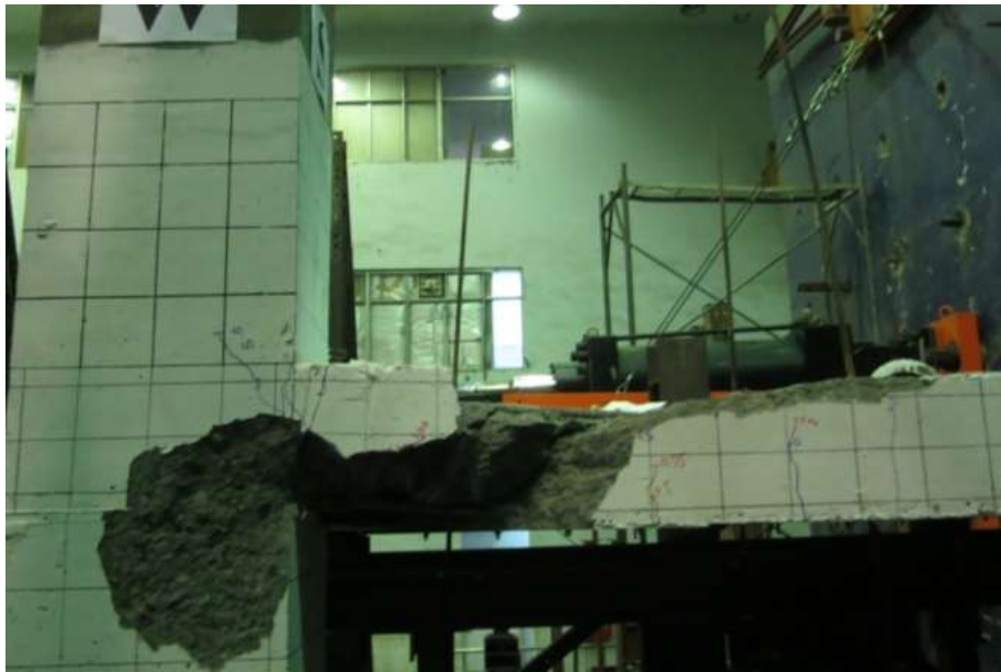
(b) After Loose Concrete Removal
