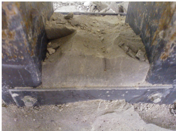
(a) Failure Mode of Web Connectors
