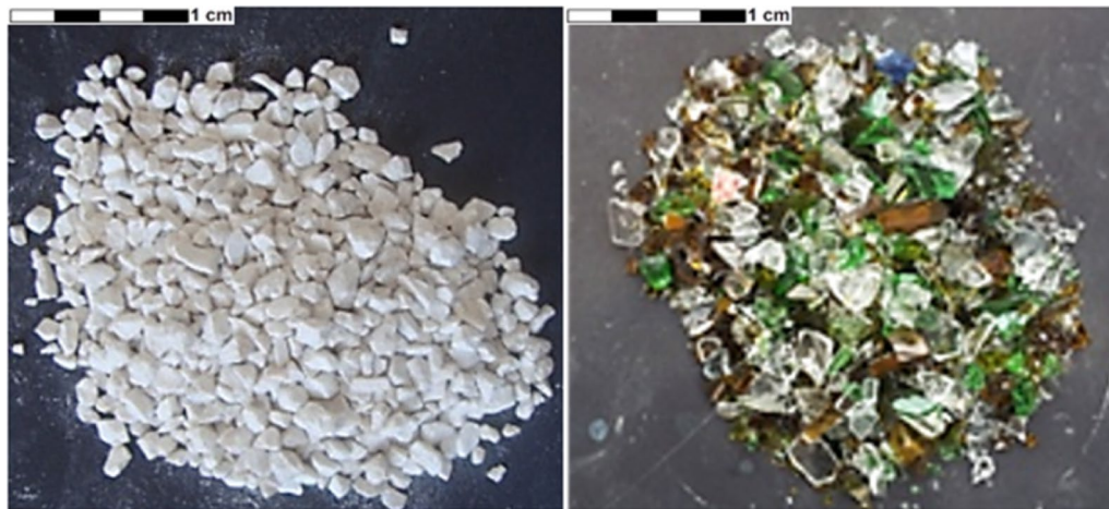
Fig. 1 Calcareous gravel (left) and recycled glass (right).
