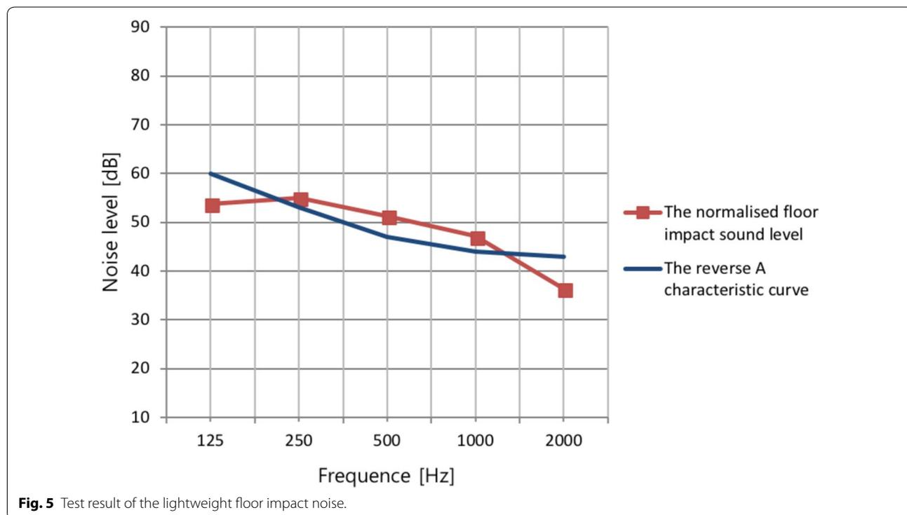
**Fig. 5** Test result of the lightweight floor impact noise.
