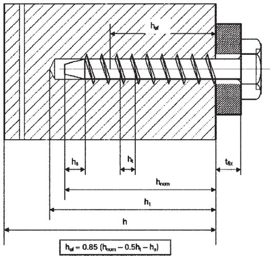
Fig. 4—Typical factors associated with embedment of concrete screw anchor.
