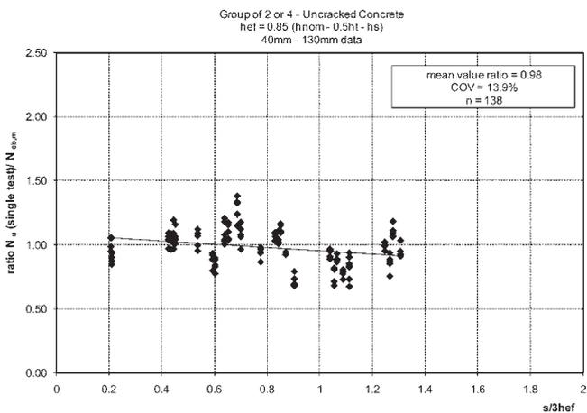
*Fig. 13—Ratio of measured to predicted strength versus spacing distance. (Note: 1 mm = 0.0394 in.)*
