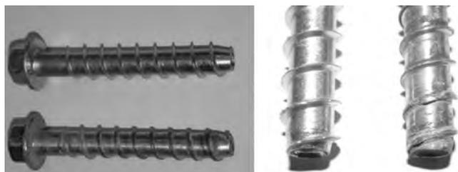
Fig. 15—Thread wear before and after installation of two types of concrete screws currently offered in the market.
