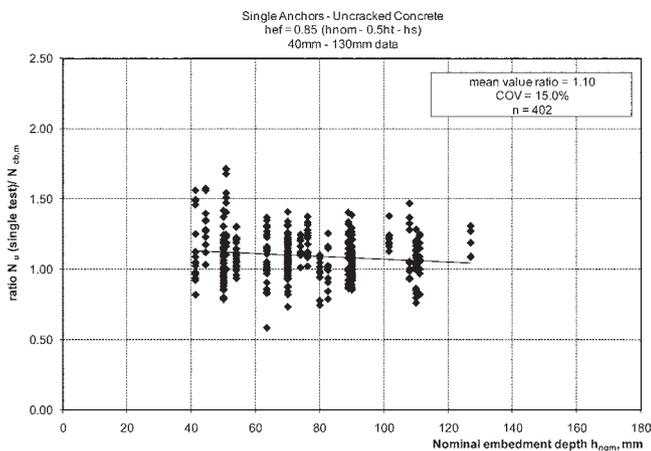
Fig. 5—Ratio of measured to predicted strength versus nominal embedment. (Note: 1 mm = 0.0394 in.)
