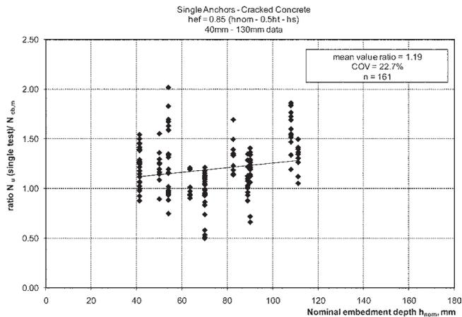
Fig. 10—Ratio of measured to predicted strength versus nominal embedment depth, 0.3 mm (0.012 in.) crack width. (Note: 1 mm = 0.0394 in.)
