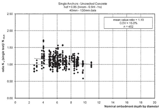
Fig. 6—Ratio of measured to predicted strength versus embedment by diameter. (Note: 1 mm = 0.0394 in.)
