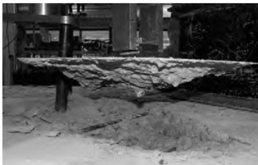
(a) Concrete cone originating near bottom of anchor
