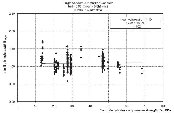
Fig. 7—Ratio of measured to predicted strength versus concrete compressive strength. (Note: 1 mm = 0.0394 in.; 1 MPa = 145 psi.)
