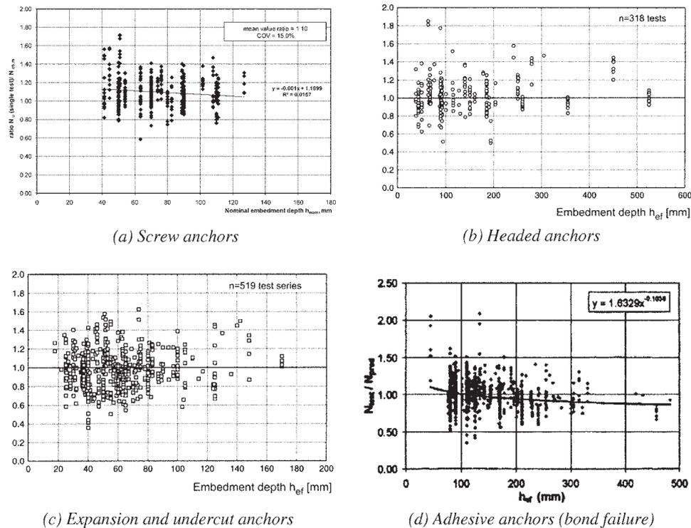
Fig. 14—Comparison of databases for various anchor types under tension loading in uncracked concrete: (a) current screw anchor database; (b) headed studs<sup>11,12</sup>; (c) expansion and undercut anchors<sup>13</sup>; and (d) adhesive anchors—bond failure.<sup>3</sup> (Note: 1 mm = 0.0394 in.)
