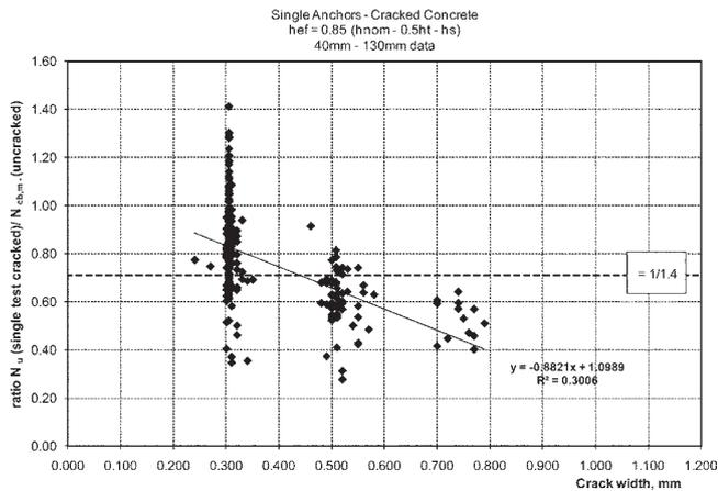
Fig. 9—Ratio of measured to predicted (uncracked) strength versus crack width. (Note: 1 mm = 0.0394 in.)
