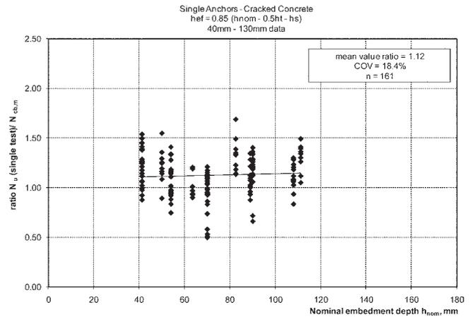
Fig. 11—Amended ratio of measured to predicted strength versus nominal embedment depth, 0.3 mm (0.012 in.) crack width. (Note: 1 mm = 0.0394 in.)
