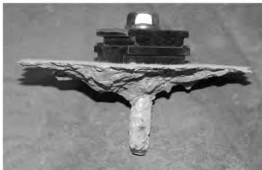
(b) Mixed failure mode of pullout and concrete cone
