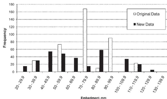
Fig. 3—Histogram of tested embedment depths from original database and additional data. (Note: 1 mm = 0.0394 in.)
