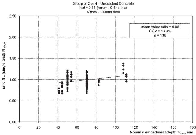
*Fig. 12—Ratio of measured to predicted strength versus embedment depth. (Note: 1 mm = 0.0394 in.)*
