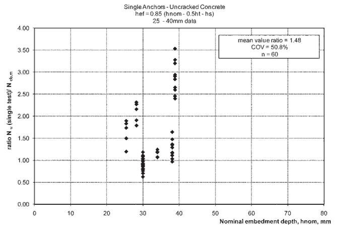
Fig. 8—Ratio of measured to predicted strength versus nominal embedment depths: shallow embedments. (Note: 1 mm = 0.0394 in.)
