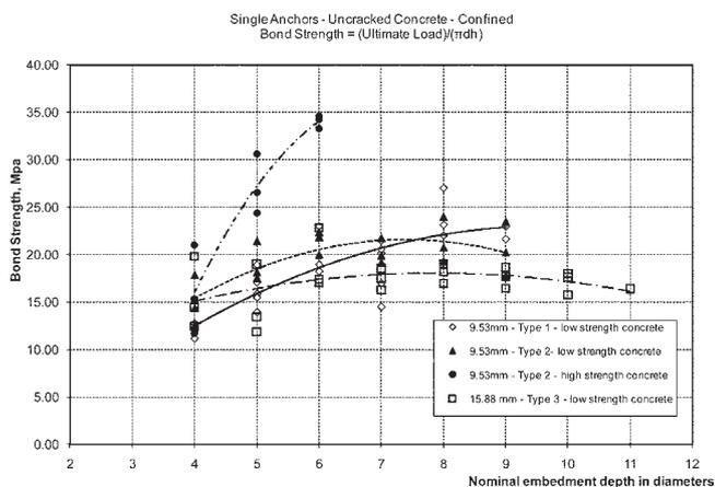
Fig. 16—Bond strength versus nominal embedment with best-fit second-order polynomial trend lines. (Note: 1 mm = 0.0394 in.; 1 MPa = 145 psi.)
