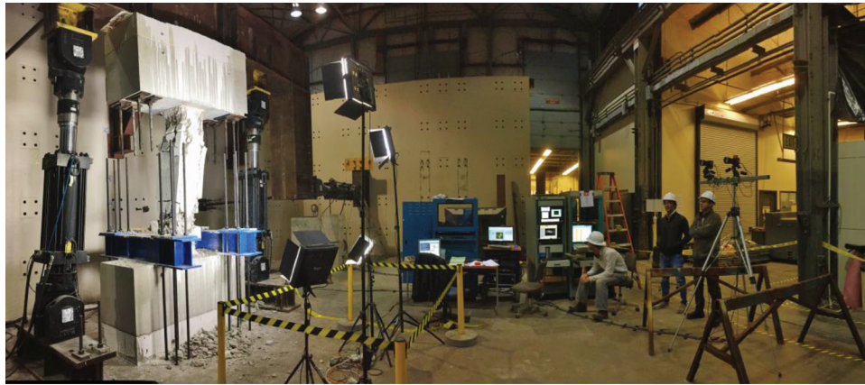
Fig. 2—Column CS100 and test setup at end of test.
