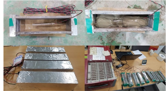
Fig. 3 Drying shrinkage test set-up.
