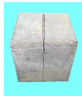
c Splitting tensile test
