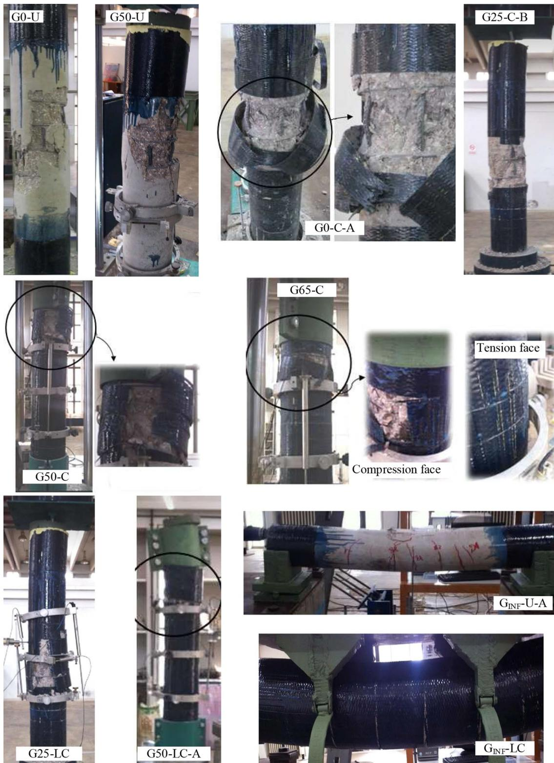
**Fig. 5** Examples of observed failure patterns in test specimens.
