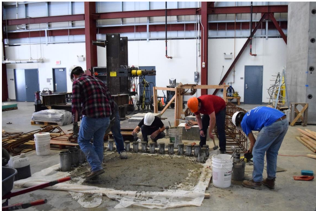
Figure 21 – Preparing concrete cylinders and in-situ tests during casting
