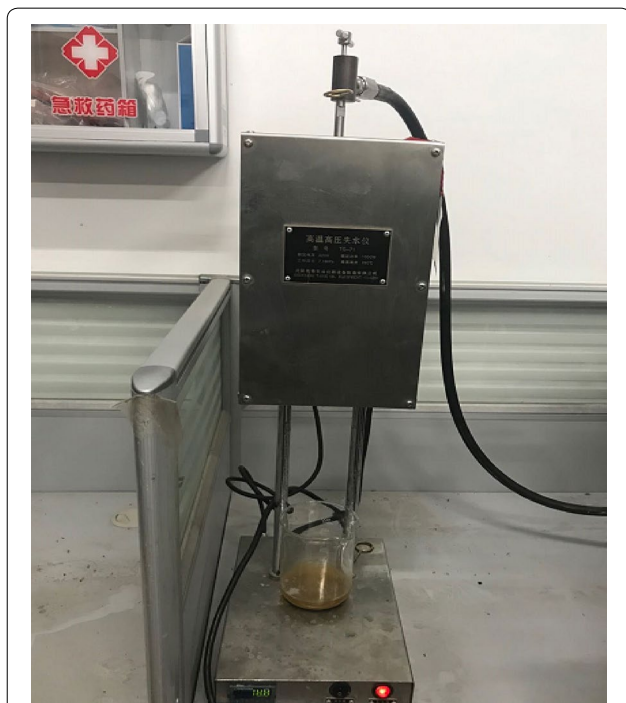
Fig. 1 TG-71 Fluid loss tester
