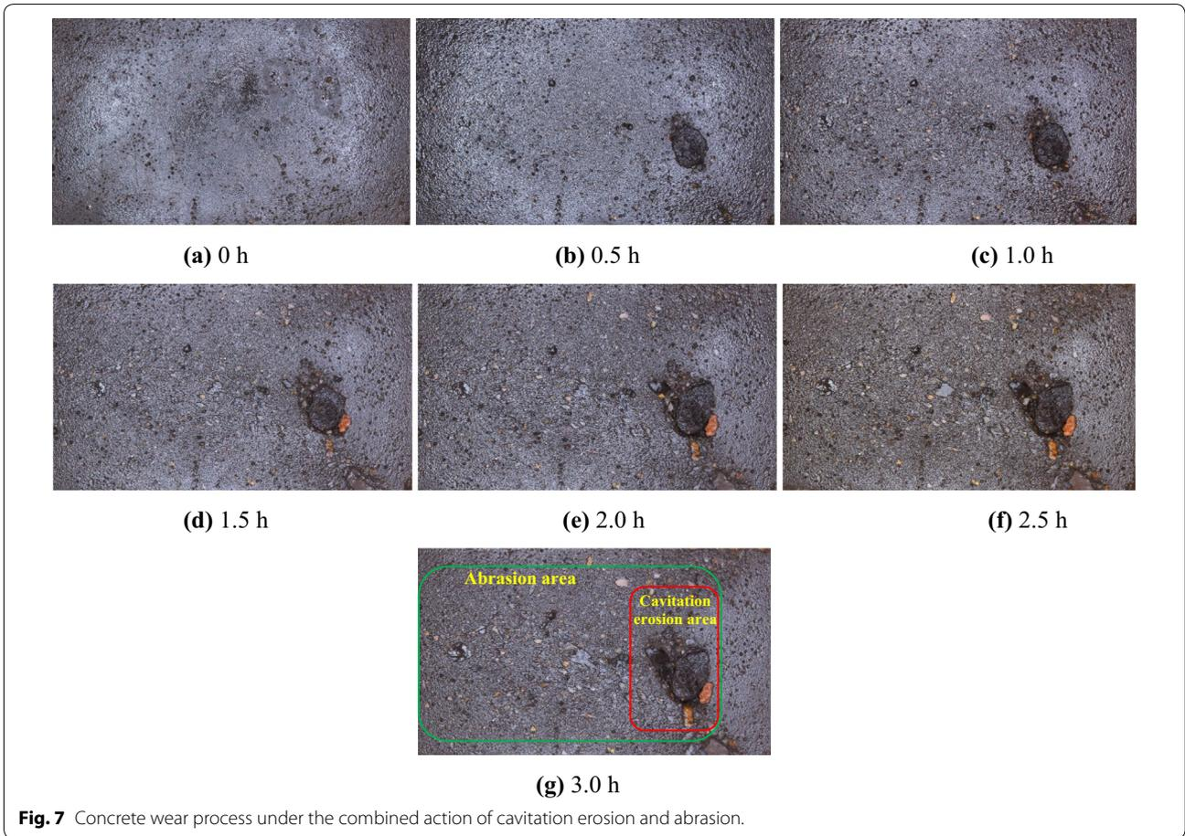
**Fig. 7** Concrete wear process under the combined action of cavitation erosion and abrasion.
