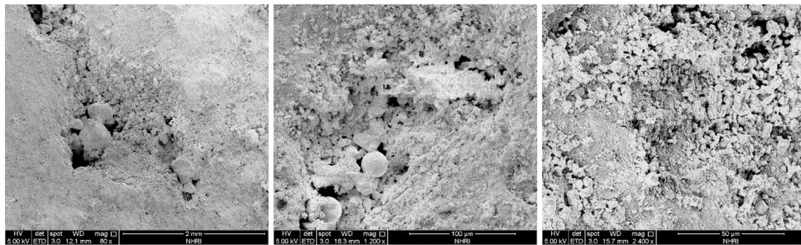
(c) After cavitation erosion only
