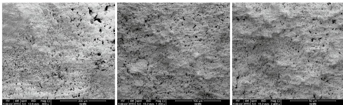
(d) After the combined action of cavitation erosion and abrasion
