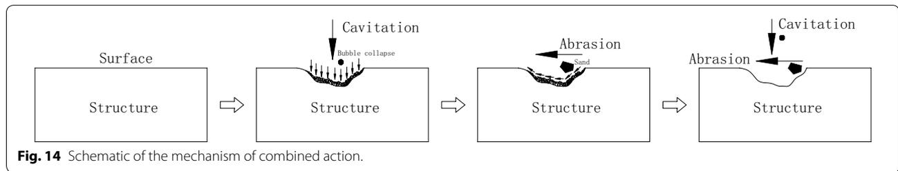
system for the combined action of cavitation erosion and abrasion was designed and constructed, and high-speed sand mixing flow only appeared in the test section. The developed experimental device could reasonably simulate the combined action of cavitation erosion and abrasion, thereby providing a valid way to investigate the mechanism of their combined action.
