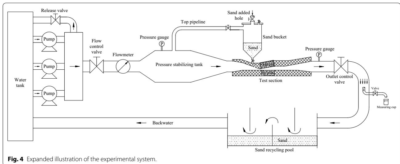
the sand content of sand mixing flow can be easily controlled, thereby laying the foundation for conducting different condition tests.
