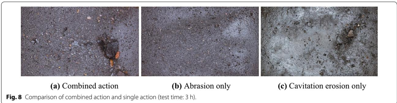
**Fig. 8** Comparison of combined action and single action (test time: 3 h).
