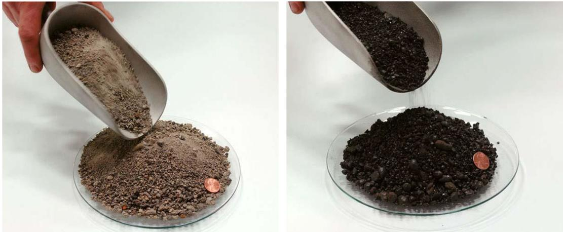
**Figure 2-13.** PC bottom ash (left) and boiler slag (right) [38]
