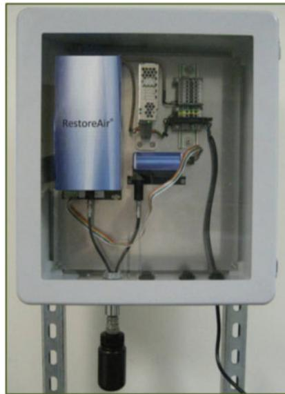
**Figure 3-5.** RestoreAir setup (Boral) – a commercial chemical passivation technology[118]
