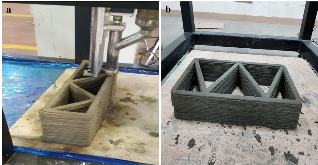
Fig. 5 a Printing of a hollow wall using the 3D printer and b printed hollow wall for functional testing of the 3D printer.
