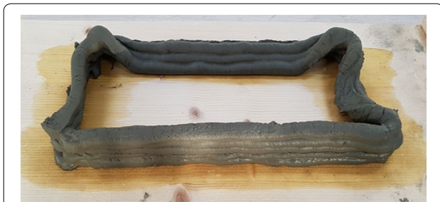
Fig. 11 Sinking deformation of layers.
