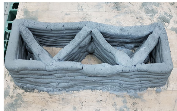
Fig. 6 Constructed hollow walls with the paste.
