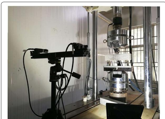
**Fig. 1** Three-point bending fracture test of concrete.
