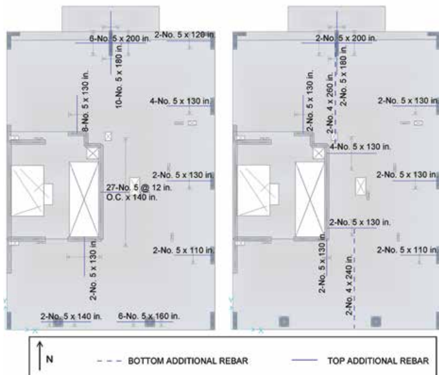
Fig. 4: Reinforcing steel for the prototype slab with Grade 60 and Grade 80 bars. Top mats comprise No. 5 bars at 12 in. on center each way. The typical top and bottom mats are indicated above each floor plan; and additional top or bottom reinforcing bars required for strength are shown on each floor plan (Note: 1 in. = 25 mm)
