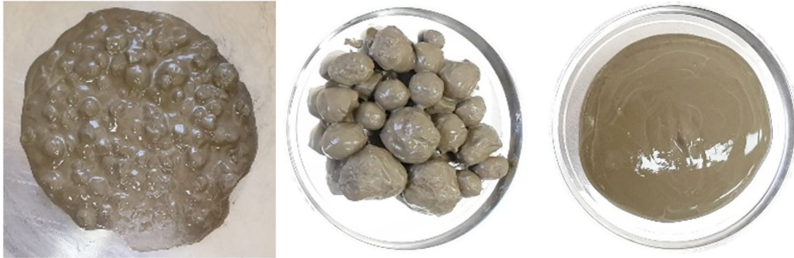
Fig. 1 LWA-paste sample, wet-sieved coarse LWA and wet-sieved paste.
