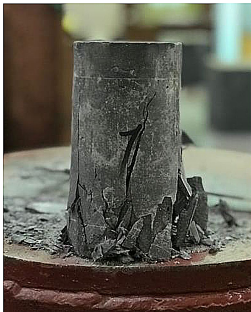
Fig. 13 Formation of cracks and UHPFRC (T3) steel fibers at failure of compression tests
