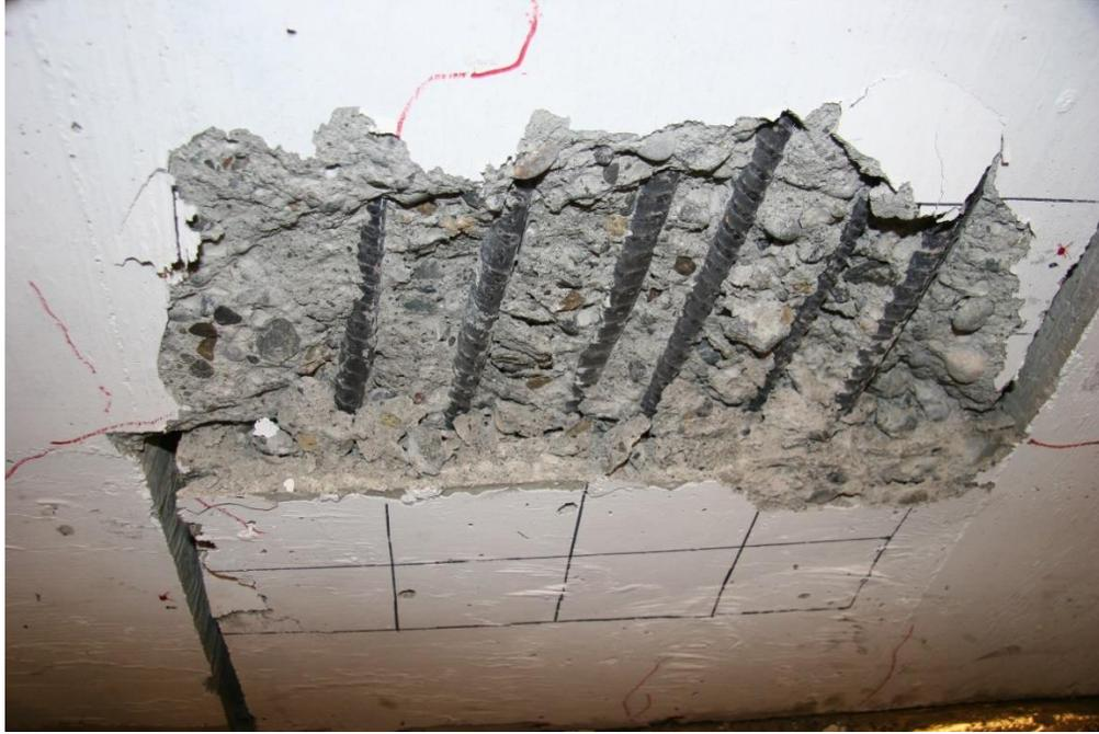
**Figure 4.28: Photograph of the revealed reinforcement after test (UW60S-12 East side).**
