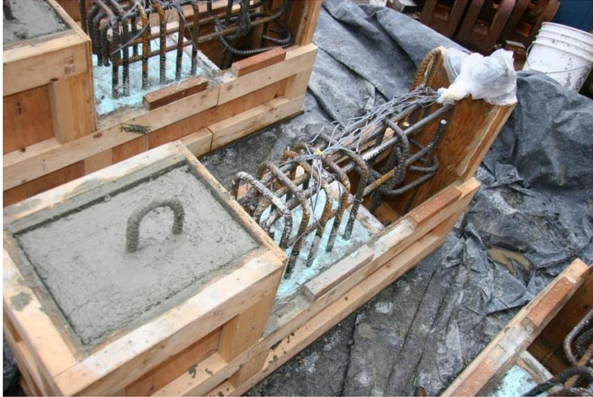
**Figure 3.4: Photograph showing the first half of the specimen being casted and the interface being treated with surface retarders.**
