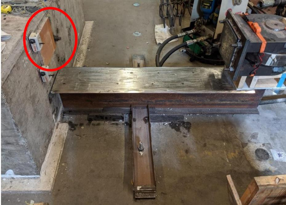
**Figure 3.11: Picture of the test setup. The wide flange beam was anchored down with two C-channels.**
