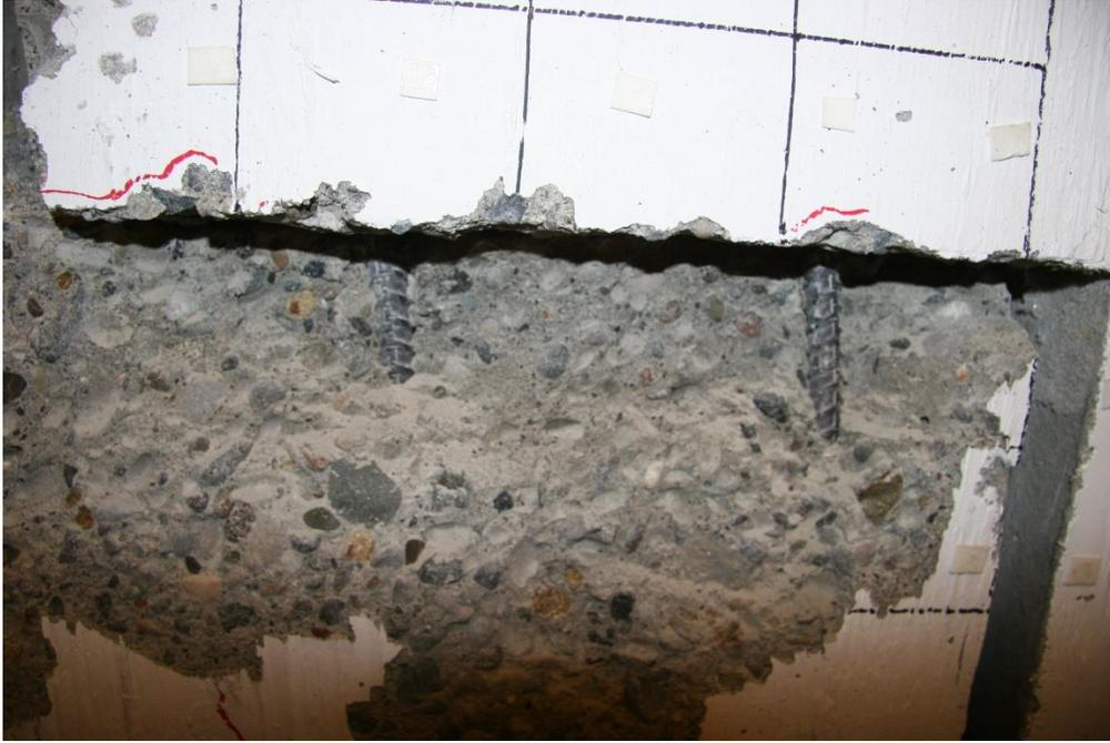
**Figure 4.52: Photograph of the revealed reinforcement after test (UW60R-4 East side).**
