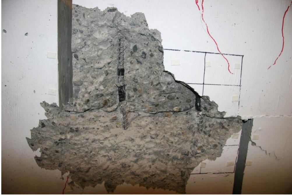
**Figure 4.69: Photograph of the revealed reinforcement after test (UW80R-4 East side).**
