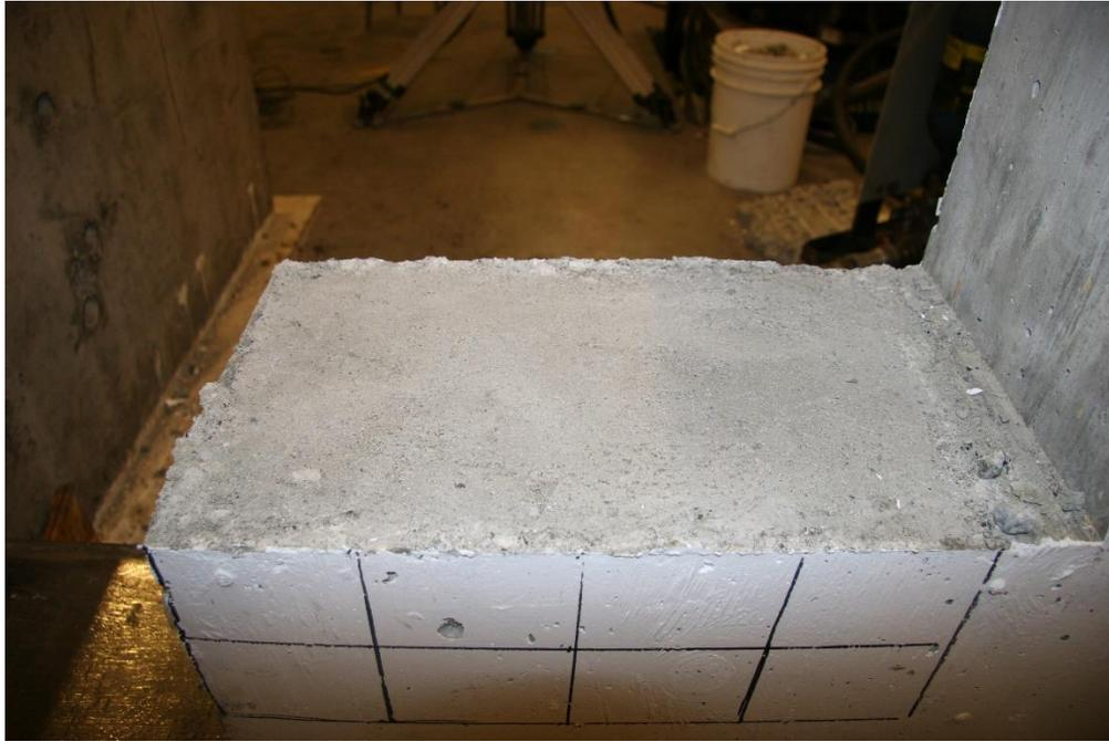
**Figure 4.3: Photograph of the interface after test (UW0S)**
