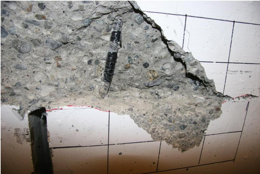
**Figure 4.53: Photograph of the revealed reinforcement after test (UW60R-4 West side).**
