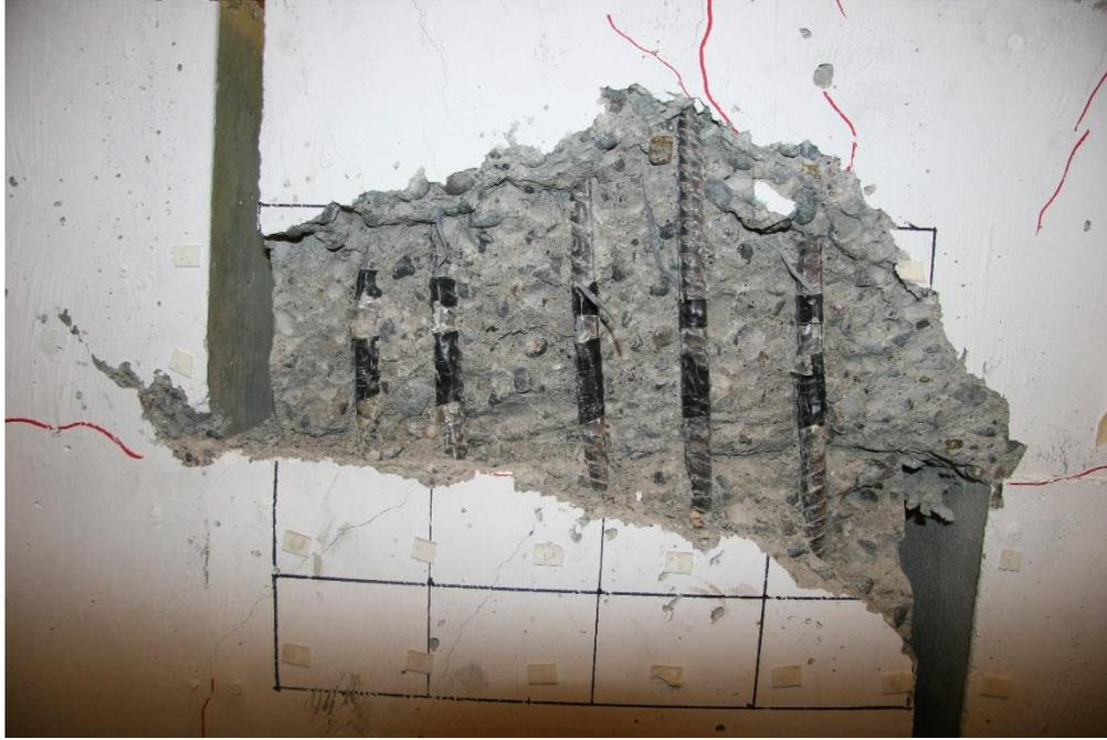
**Figure 4.78: Close up of the revealed reinforcement after test (UW80R-10 East side).**
