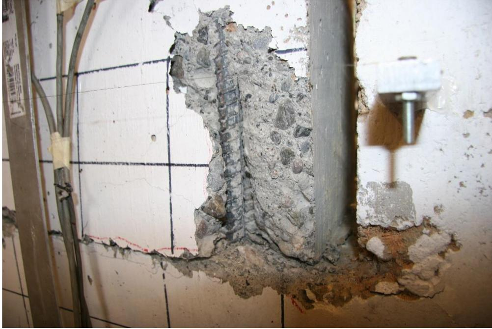
**Figure 4.39: Close up of the revealed reinforcement after test (UW80S-6 West side).**
