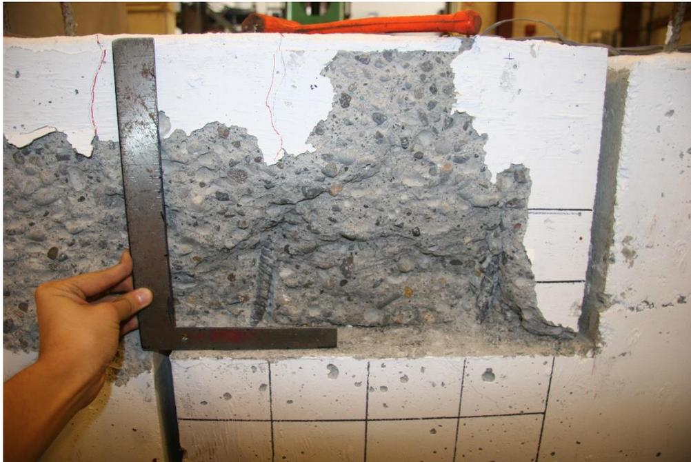
Figure 4.36: Close up of the revealed reinforcement after test (UW80S-4 West side).
