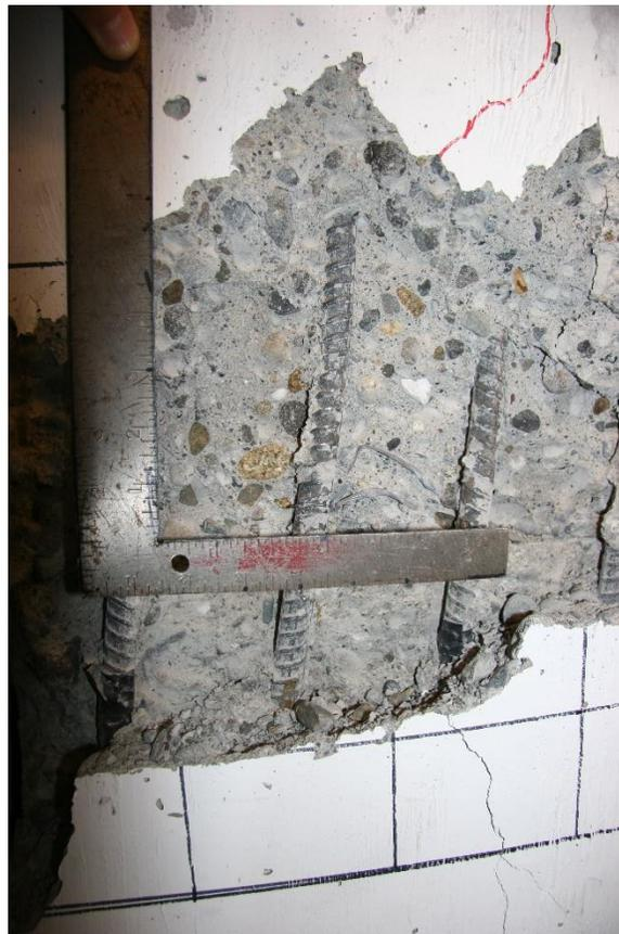
**Figure 4.43: Photograph of the revealed reinforcement after test (UW80S-8 West side).**
