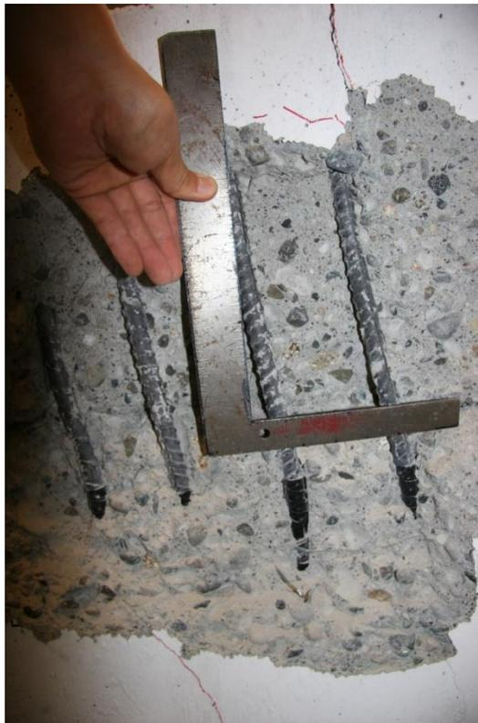
Figure 4.22: Close up of the revealed reinforcement after test (UW60S-8 West side).
