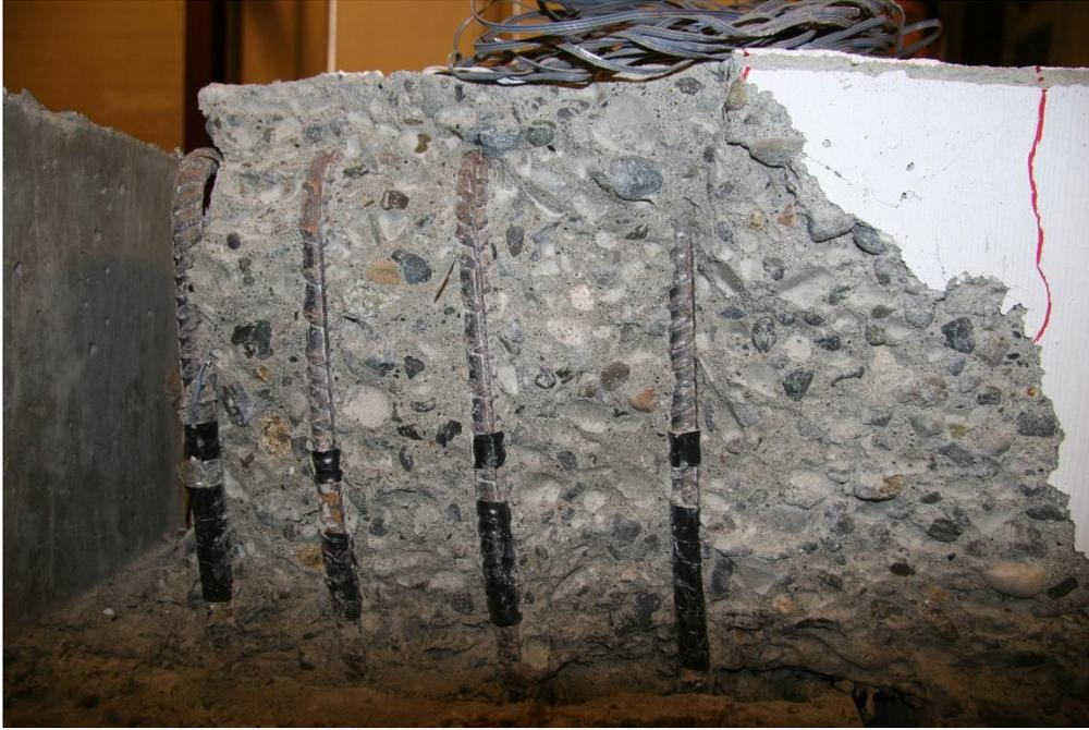
**Figure 4.75: Close up of the revealed reinforcement after test (UW80R-8 East side).**
