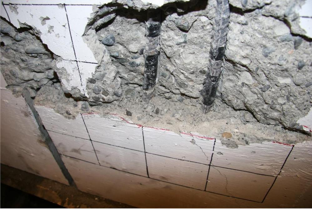
**Figure 4.56: Close up of the revealed reinforcement after test (UW60R-6 West side).**
