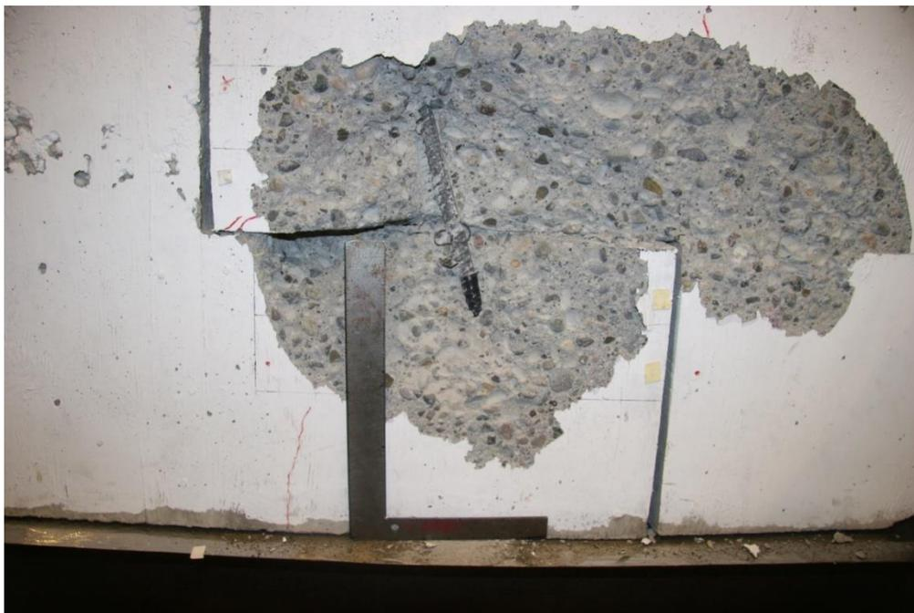
**Figure 4.10:** Close up of the revealed reinforcement after test (UW60S-2 East side).
