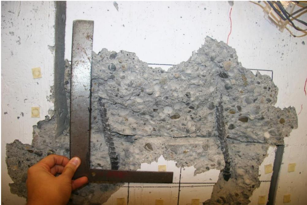
**Figure 4.14: Close up of the revealed reinforcement after test (UW60S-4 West side).**
