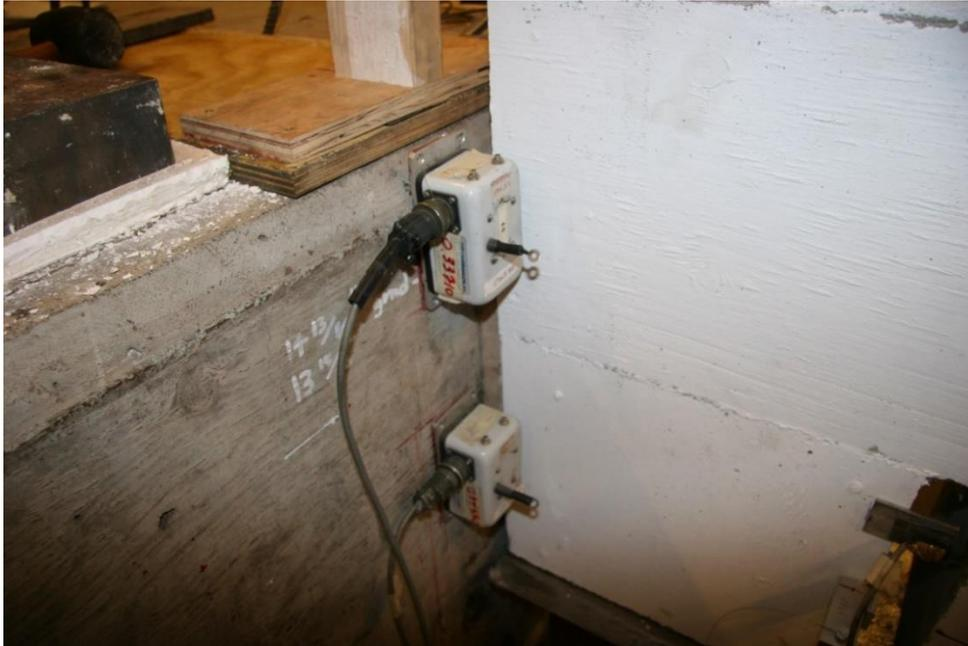
**Figure 3.14: String potentiometer attached to the reaction block**
