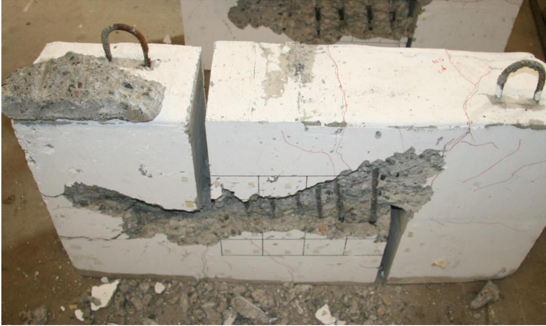
**Figure 4.49: Photograph of the revealed reinforcement after test (UW80S-12 East side).**
