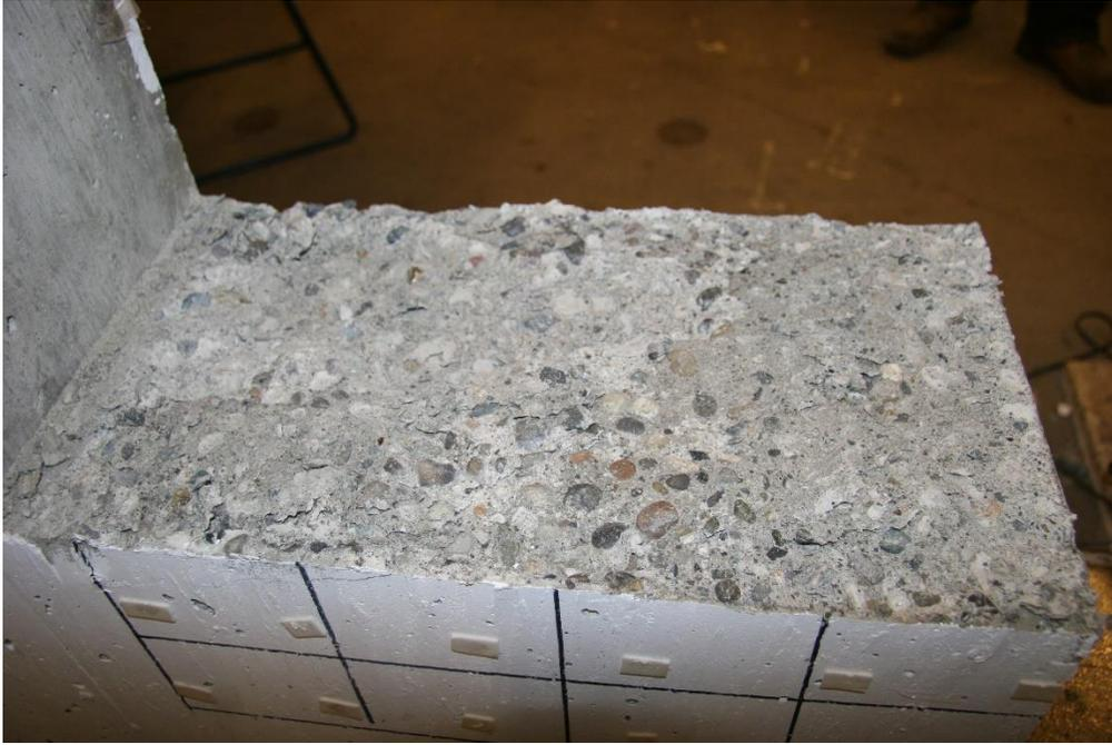
**Figure 4.6: Photograph of the interface after test (UW0R)**
