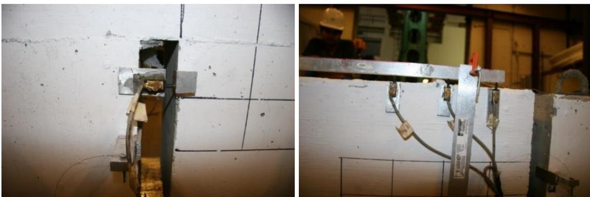
**Figure 3.15: Duncan potentiometers used during the test.**
