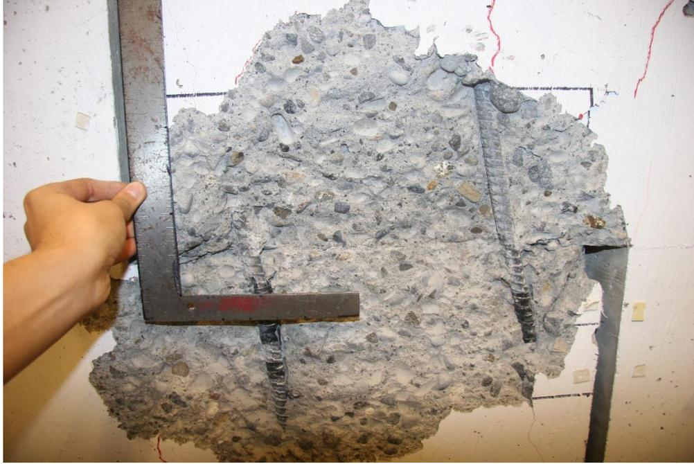
Figure 4.35: Close up of the revealed reinforcement after test (UW80S-4 East side).
