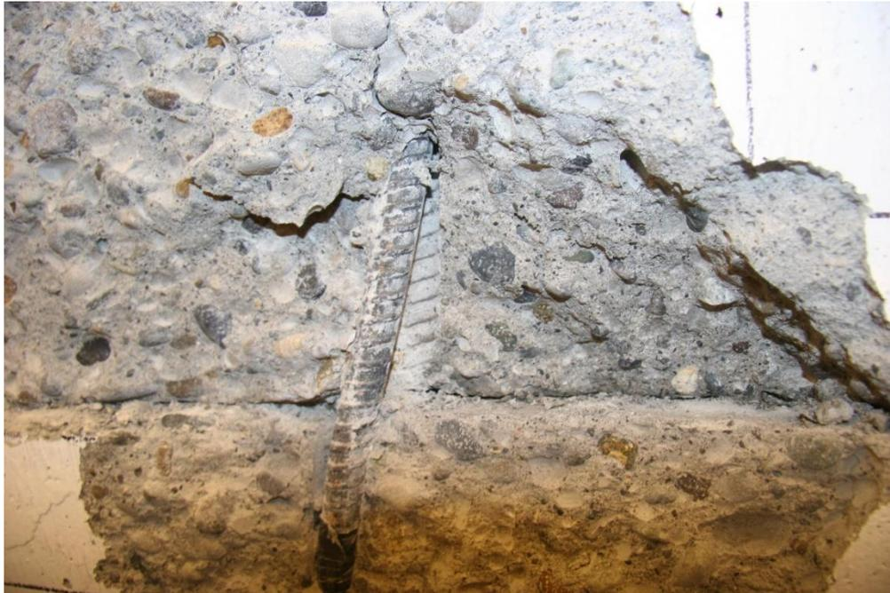
**Figure 4.9:** Close up of the revealed reinforcement after test (UW60S-2 West side).
