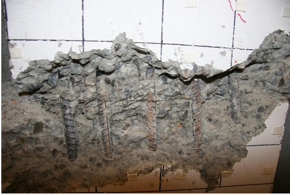
Figure 4.63: Close up of the revealed reinforcement after test (UW60R-10 East side).
