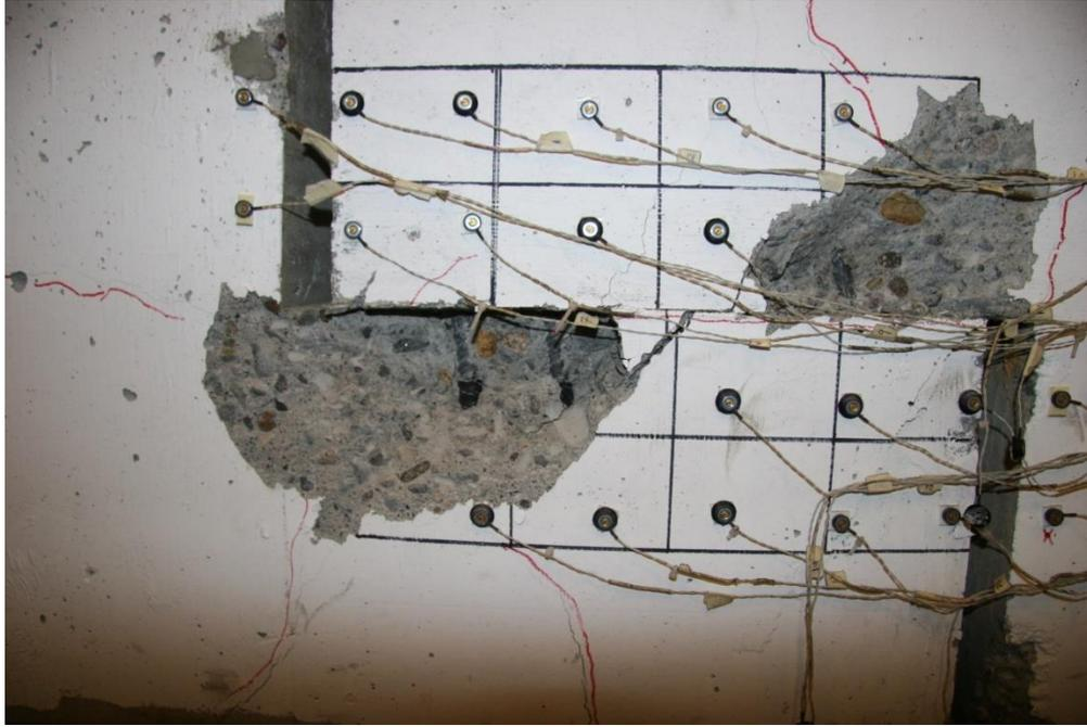
Figure 4.25: Photograph of the revealed reinforcement after test (UW60S-10 East side).
