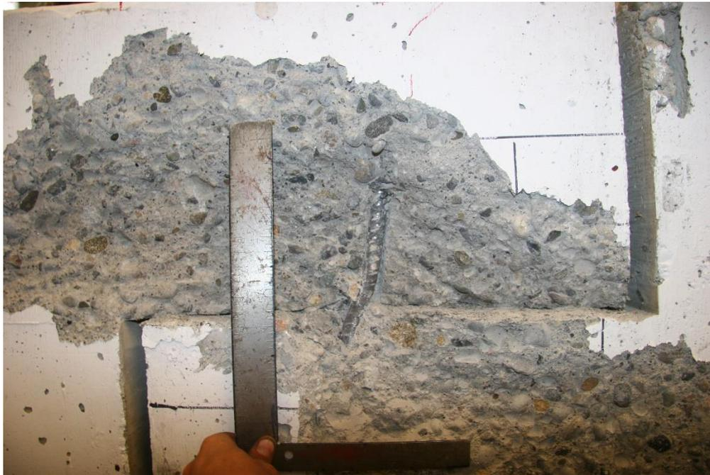
**Figure 4.32: Close up of the revealed reinforcement after test (UW80S-2 West side).**
