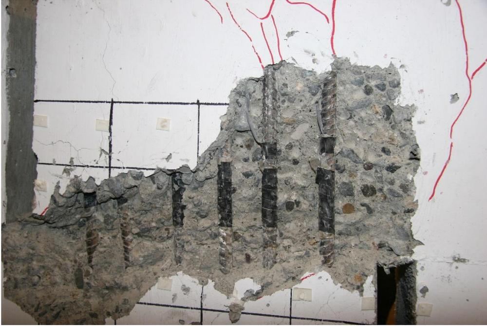
**Figure 4.81: Close up of the revealed reinforcement after test (UW80R-12 East side).**
