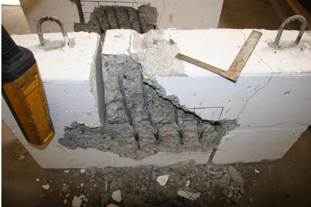
**Figure 4.42: Close up of the revealed reinforcement after test (UW80S-8 East side).**
