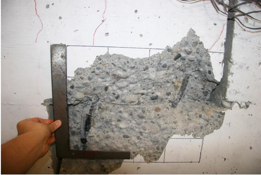
**Figure 4.13: Close up of the revealed reinforcement after test (UW60S-4 East side).**
