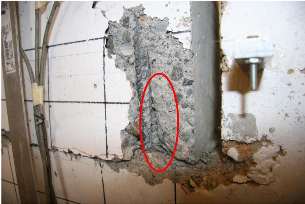
Figure 5.10: Close up of the revealed reinforcement after test (UW80S-6 West side).
