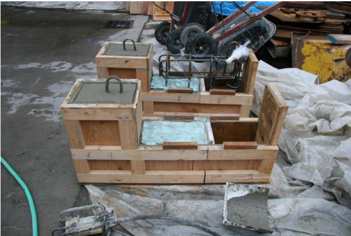
**Appendix A-9: Photograph of UW60R-4 and UW0R after first half was cast. The interfaces were treated with retarders.**
