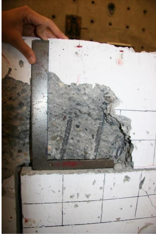
Figure 4.21: Close up of the revealed reinforcement after test (UW60S-8 East side).
