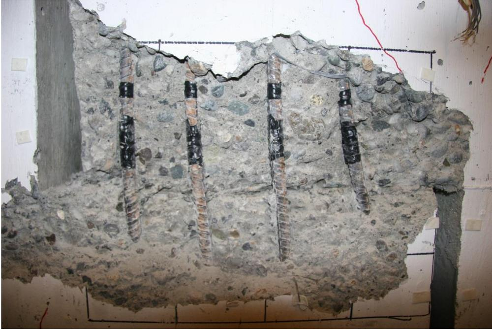
Figure 4.60: Close up of the revealed reinforcement after test (UW60R-8 East side).
