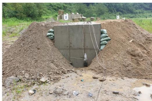
(a) Normal strength concrete structure before explosion
