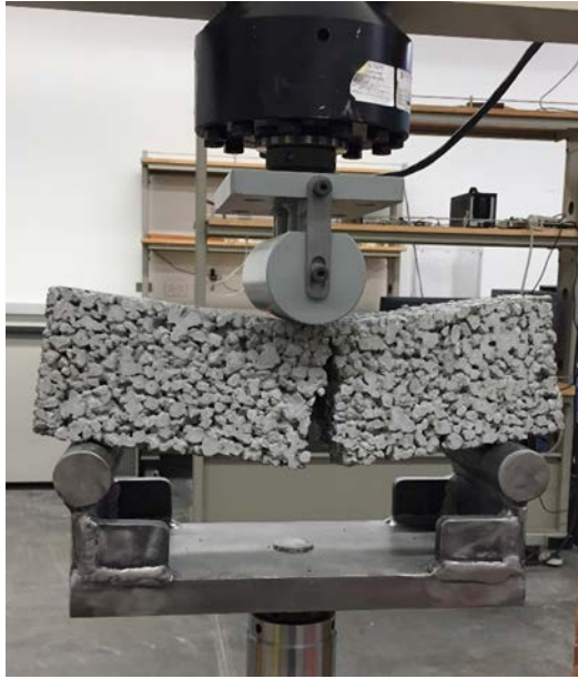
Fig. 2 Beam failure after cyclic flexural fatigue loading
