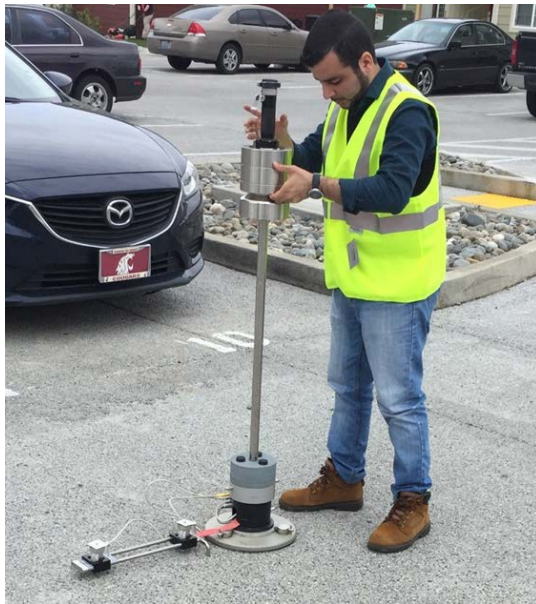
Fig. 4 LWD testing conducted on PC pavement
