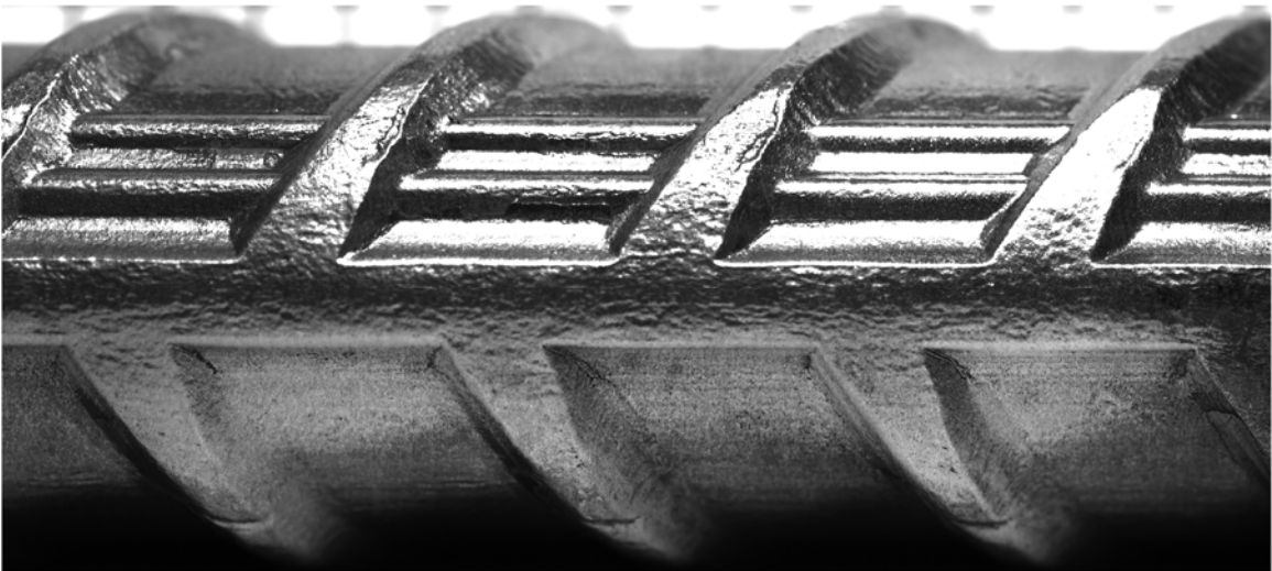
Figure 2-4: Front view of longitudinal geometry for M1-B2-100-#8
