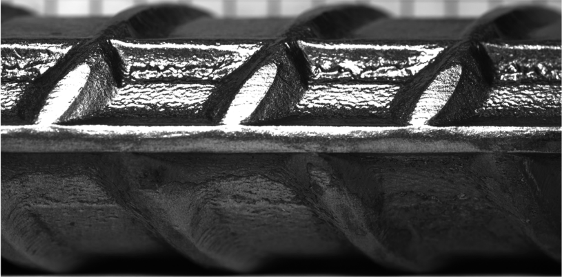
Figure 2-3: Front view of longitudinal geometry for M1-B2-80-#8
