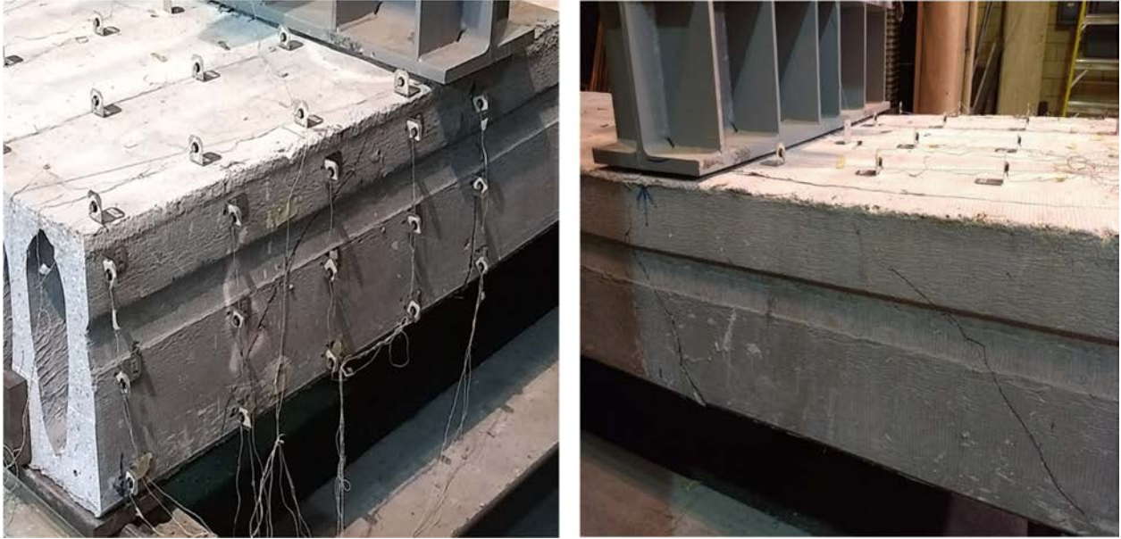
Figure 16 - Typical web cracking for test spans in Series 2 with external prestressing
