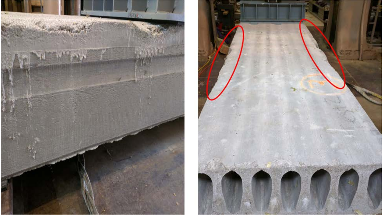
Figure 7 – Flange defects in a slab manufactured using a slip-form process
