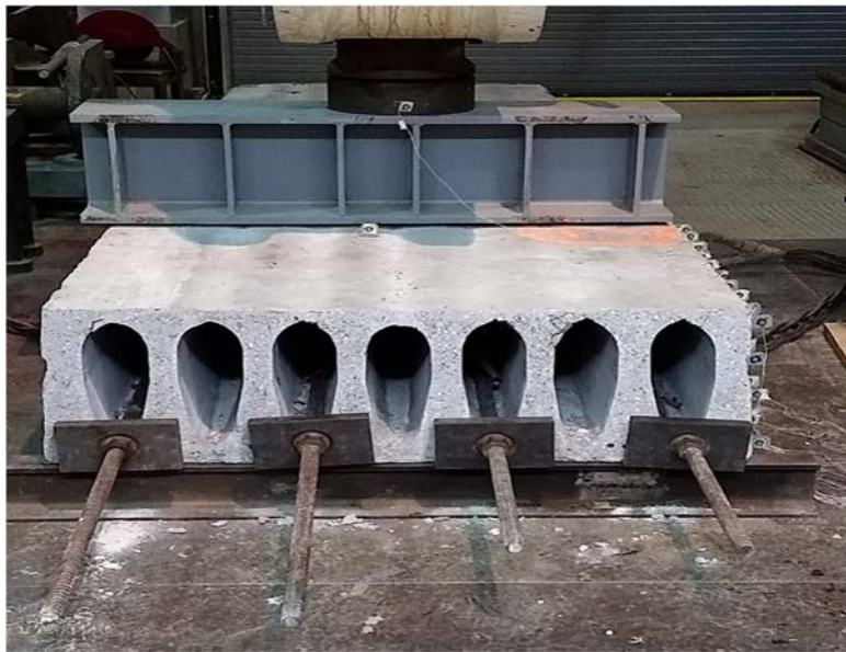
Figure 8 - External prestressing applied to hollow-core slabs in Series 2
