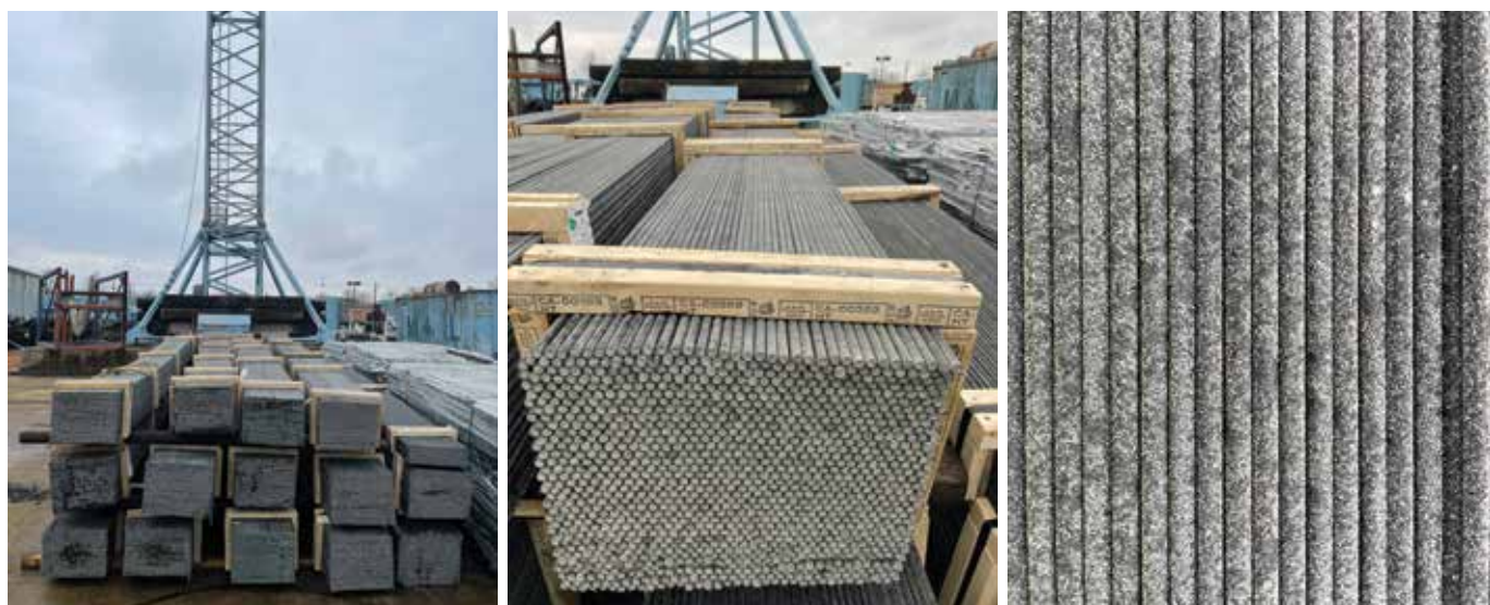
Fig. 1: BFRP bars used to reinforce topping slabs
