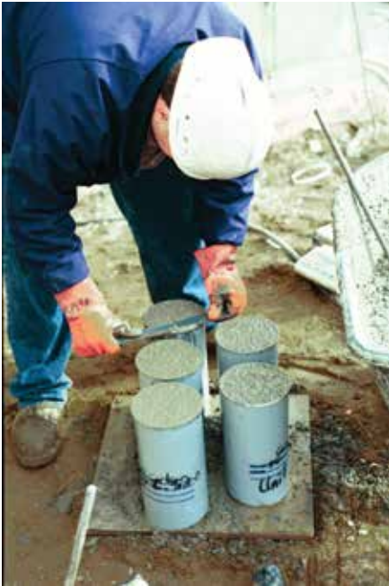
Fig. 1: Typically, four to six 6 x 12 in. concrete cylinders are cast at the jobsite to fulfill project specification requirements (photo courtesy of PCA)
