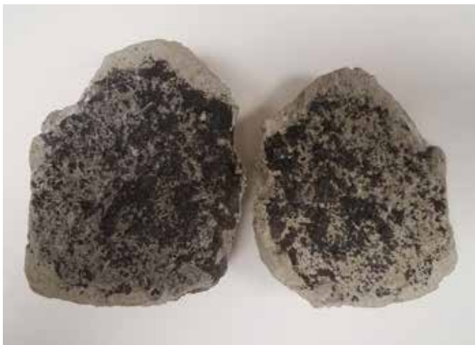
Fig. 3: An X-PHALT repair on asphalt. The sample was subjected to cleavage at the interface, exhibiting pullout failure, thus indicating good bond
