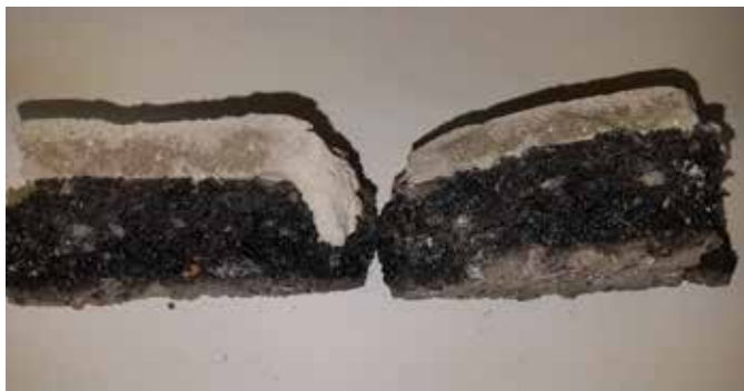
Fig. 2: An X-PHALT overlay on asphalt. The sample was subjected to bending and fractured in flexure with zero delamination
