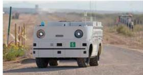
The Honda AWV combines the company's rugged and durable off-road side-by-side platform with emerging advanced autonomous technology. The result is a new category of capable work vehicle that can be deployed in a variety of dynamic work environments. The Honda AWV employs a suite of sensors to operate autonomously, using GPS for location, radar and lidar for obstacle detection, and stereoscopic cameras for remote monitoring. The vehicle can also be operated by remote control.
