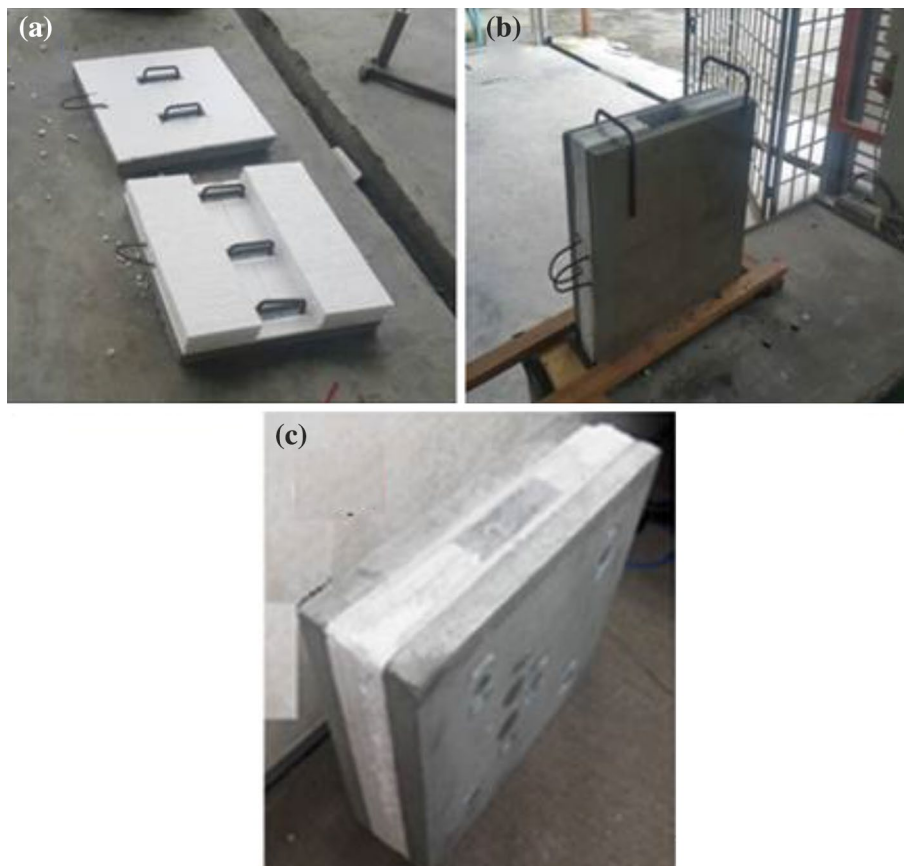
Fig. 3 Construction process: a insulation, b assembling and c completed panel.
