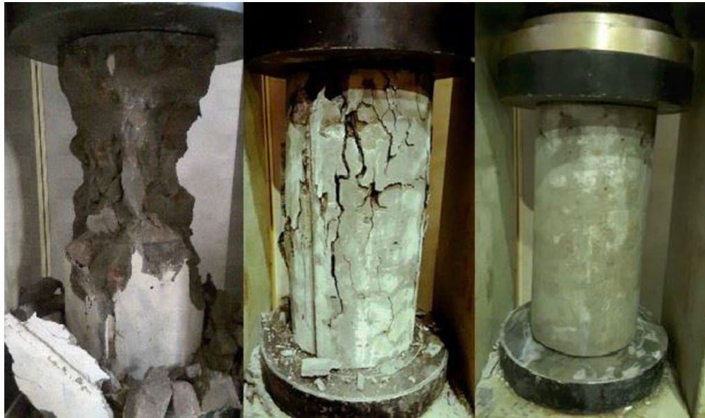
Fig. 12 PAC cylindrical specimens under uniaxial compressive load: (Right) cylindrical specimen, (Middle) crack growth during loading, (Left) failure.
