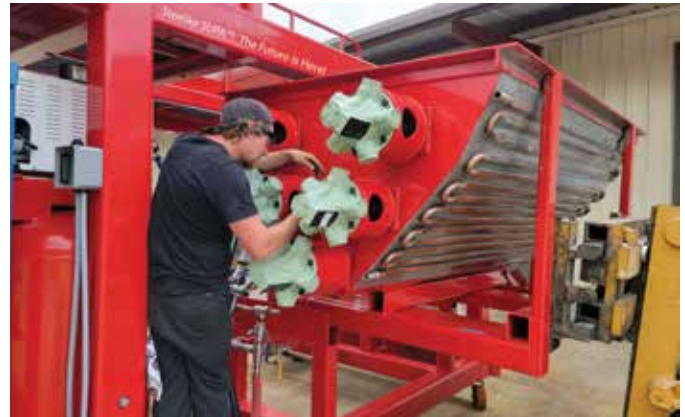
The Steelike SUPA mixer able to pump Steelike UHPC
