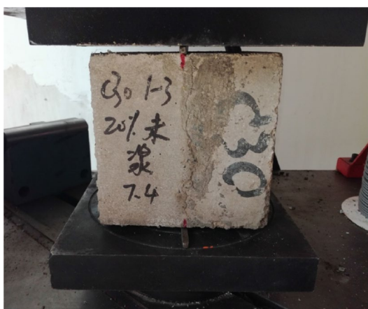
Fig. 6 Photograph of the splitting tensile strength test setup for bonding tensile strength analysis.
