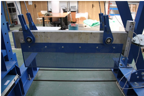
Fig. 3 The measuring attachment of the impactor.
