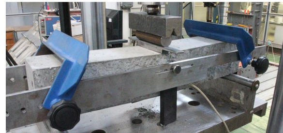
Fig. 11 The three-point bending experiment for the quasi-static testing.
