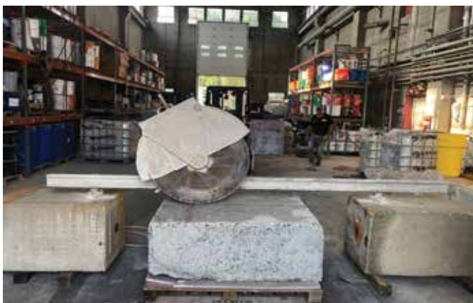
Fig. 2: BCSA runway slab sample is prepared for cutting at the CTLGroup’s laboratory
