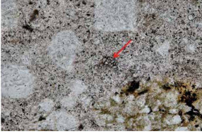
Fig. 6: Thin-section micrograph of hardened BCSA concrete, taken using a plain-polarized light source. The field of view is 0.03 in. (0.76 mm) across. Almost complete hydration is observed. The red arrow indicates a trace of residual calcium sulfoaluminate cement in the paste
