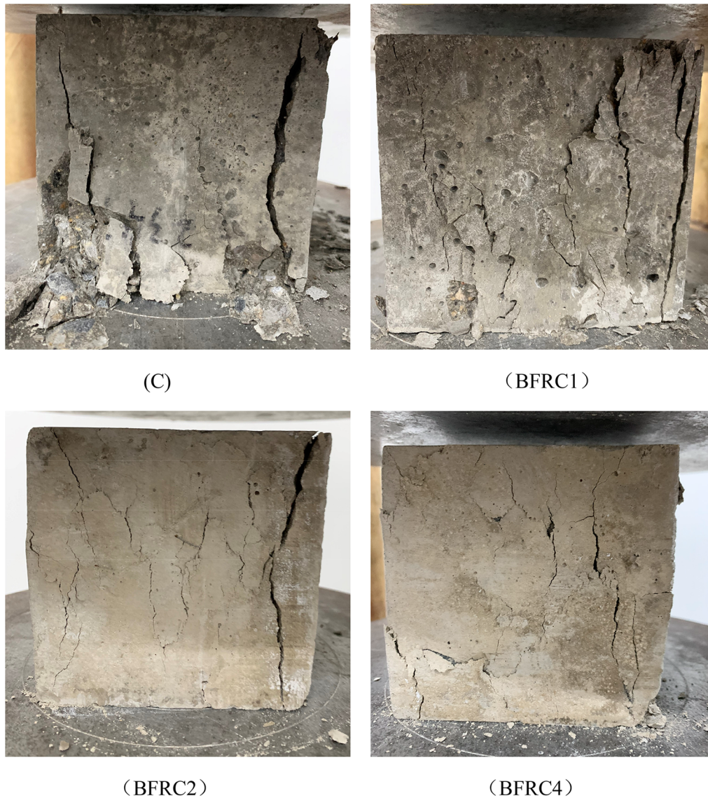
Fig. 6 Concrete compression failure pattern.
