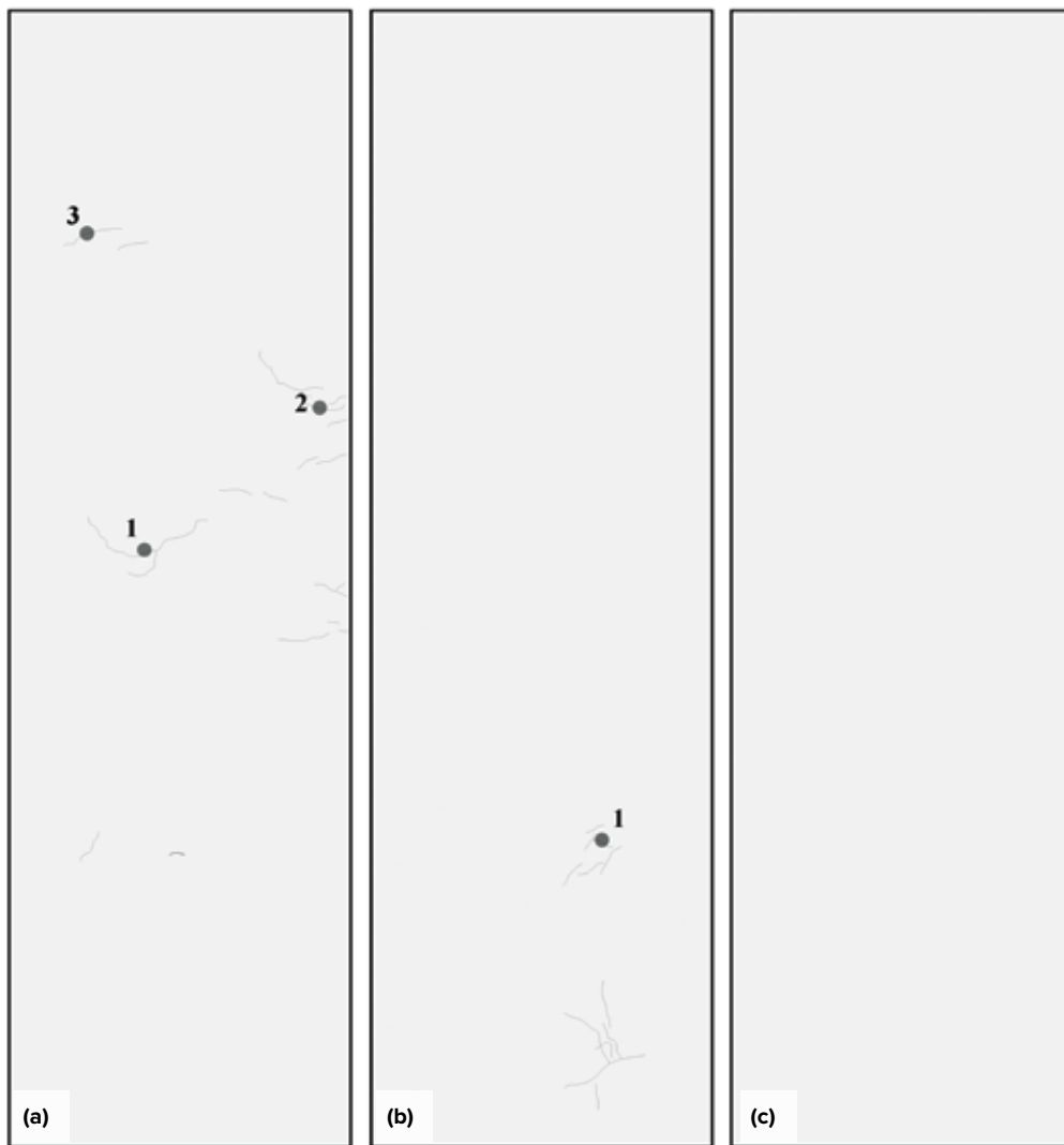
Fig. 7: Outdoor slabs crack pattern after 210 days: (a) No. 4 steel bars at 18 in. o.c.; (b) No. 4 GFRP bars at 18 in. o.c.; and (c) No. 3 GFRP bars at 18 in. o.c. (Note: Thin lines represent microcracks; and dots represent reference measuring points)
