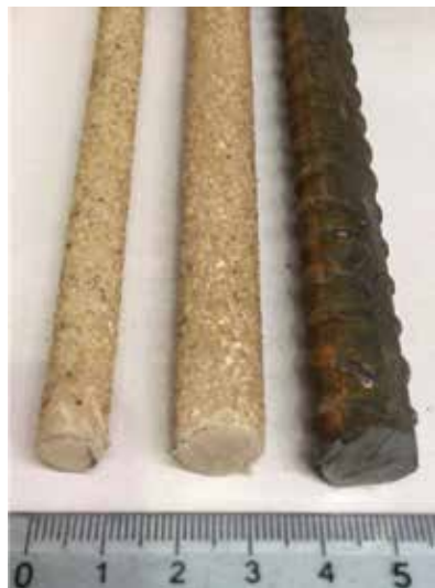
Fig. 3: Bar types used in the study, from left: No. 3 and No. 4 GFRP bars and No. 4 steel bar
