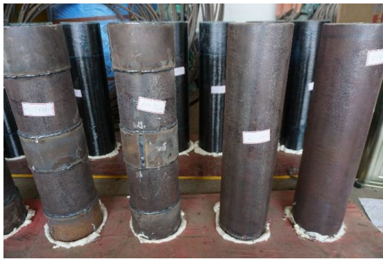
(a) Fix on the bottom formwork
