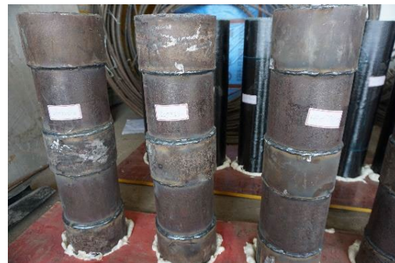
(f) CFST columns confined by steel strip
