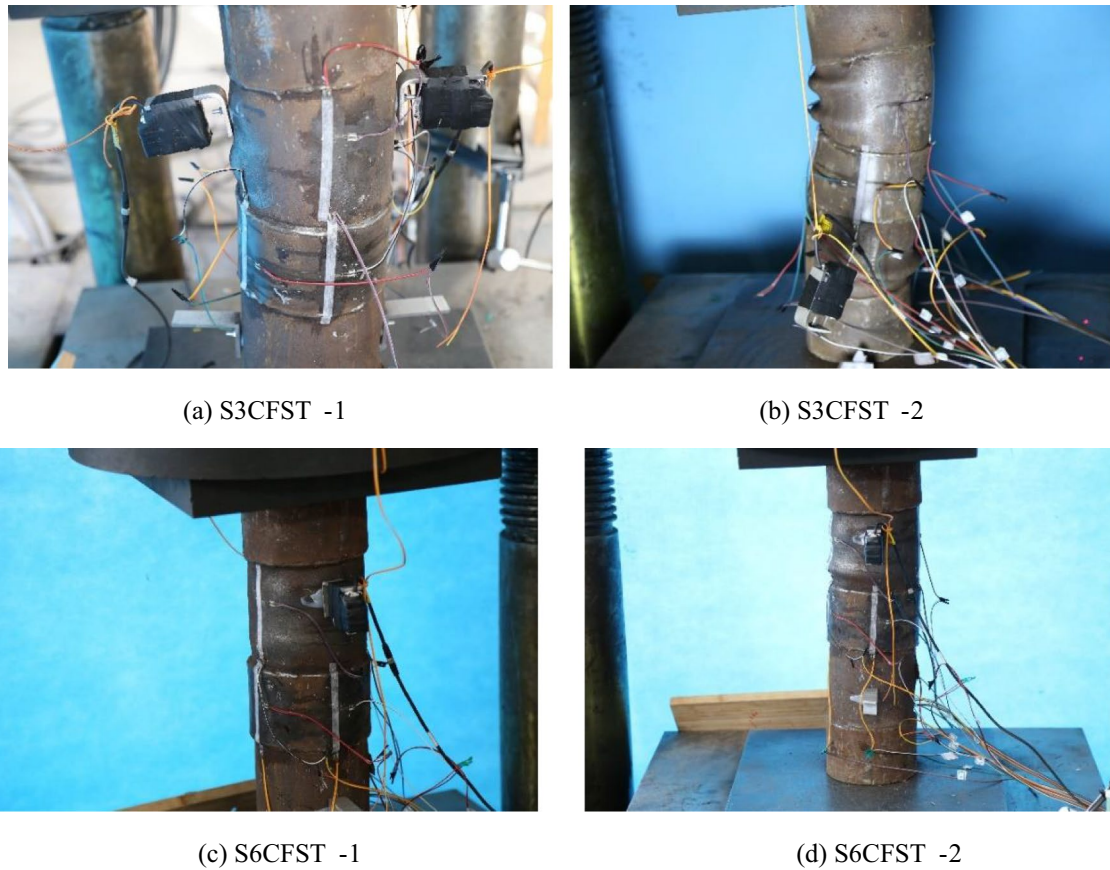
Fig. 10 Failure mode of welded steel strip-strengthened CFST columns
