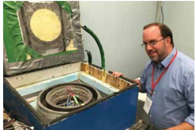
Brock Hedegaard checks out a double-ring concrete shrinkage test at the Turner-Fairbank Highway Research Center laboratory in McLean, VA, USA (photo courtesy of Brock Hedegaard)
