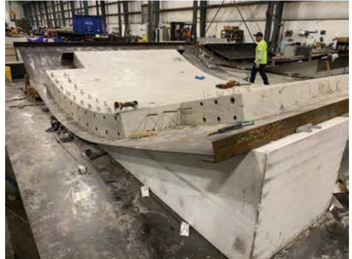
Fig. 5: Installation of reinforcement grids in a curved panel (left) and the panel after casting (right)
